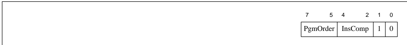
Figure 4.8 TF2 (Trace Format 2 Multi-Pipe)
