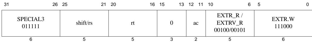
Figure 5.8 SPECIAL3 Encoding Example for EXTR.W Instruction Sub-class Type 1
