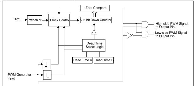
Figure 14-18: Dead Time Insertion Diagram
