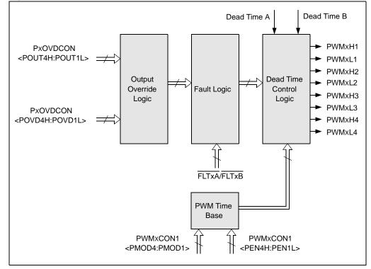
All control bits associated with the PWM output override function are in the PxOVDCON register. The upper half of the PxOVDCON register contains eight PWM Output Override bits (POVDx) that determine which PWM I/O pins will be overridden. The lower half of the PxOVDCON register contains eight PWM Manual Output bits (POUTx) that determine the state of the PWM I/O pin when it is overridden with the POVDx bit.
