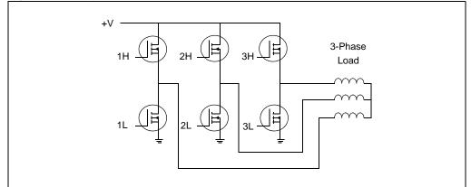
Complementary PWM Output mode is selected for each PWM I/O pin pair by clearing the PWM I/O Pair Mode bit (PMOD) in the PWM Control Register 1 (PWMxCON1<11:8>). The PWM I/O pins are set to Complementary PWM Output mode by default on a device Reset.
