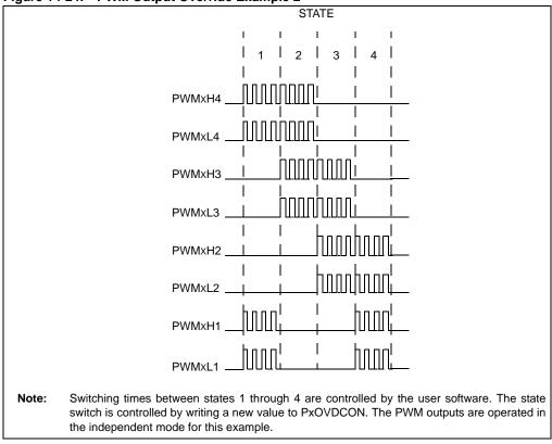
Figure 14-24: PWM Output Override Example 2
