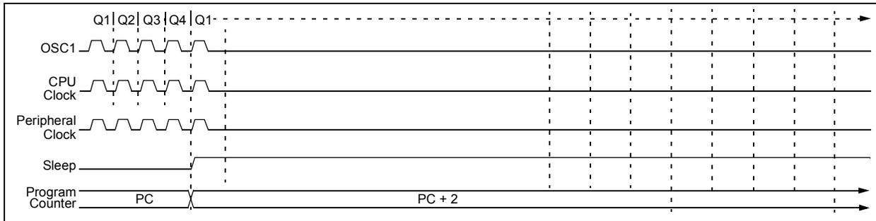
**FIGURE 4-5: TRANSITION TIMING FOR WAKE FROM SLEEP (HSPLL)**
