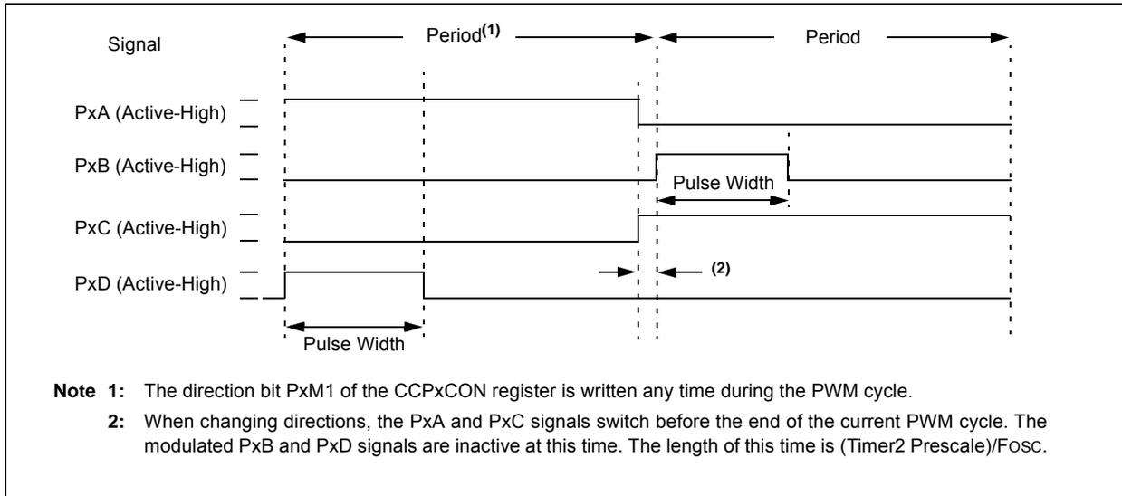
**FIGURE 15-13: EXAMPLE OF PWM DIRECTION CHANGE AT NEAR 100% DUTY CYCLE**
