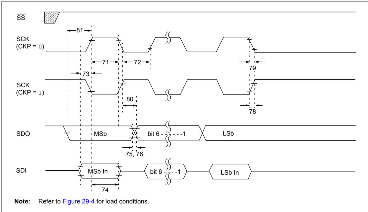
**FIGURE 29-13: EXAMPLE SPI SLAVE MODE TIMING (CKE = 0)**
