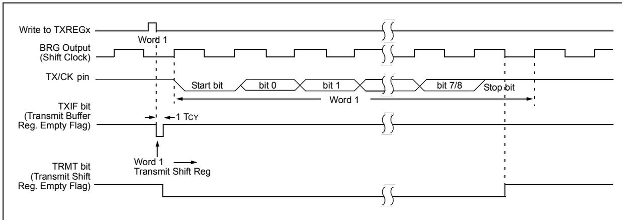
**FIGURE 17-4: ASYNCHRONOUS TRANSMISSION (BACK-TO-BACK)**
