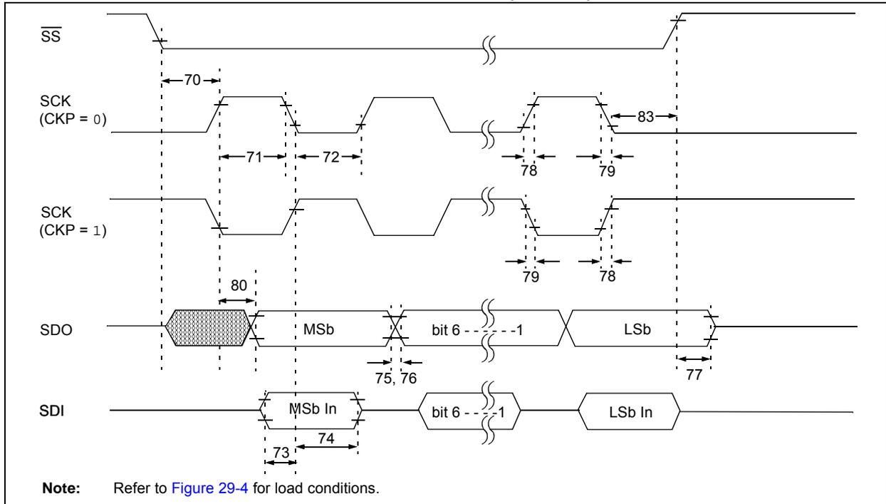
**TABLE 29-15: EXAMPLE SPI MODE REQUIREMENTS (SLAVE MODE TIMING, CKE = 0 OR 1)**
