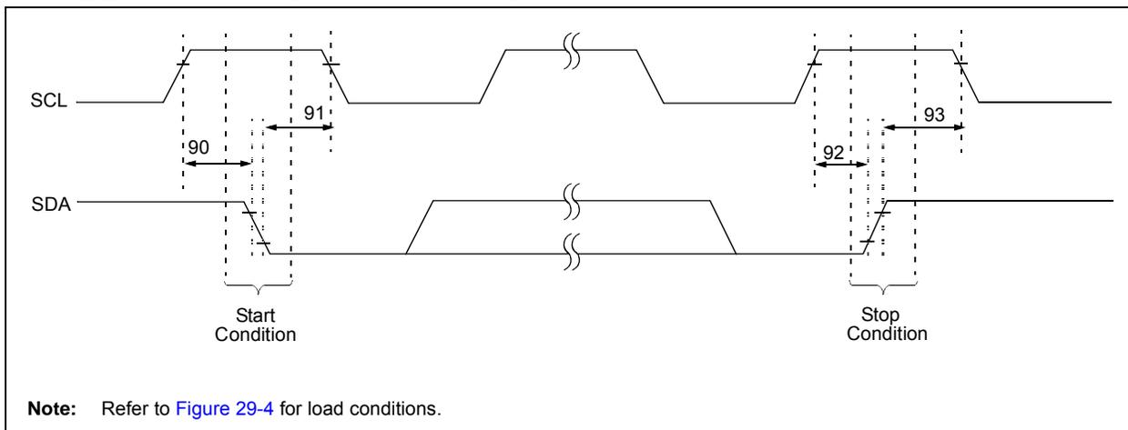
**TABLE 29-16: I<sup>2</sup>C™ BUS START/STOP BITS REQUIREMENTS (SLAVE MODE)**
