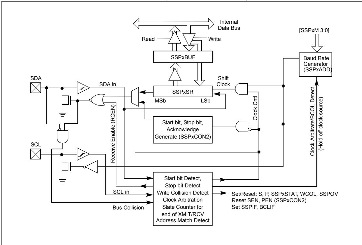
**FIGURE 16-3: MSSP BLOCK DIAGRAM (I<sup>2</sup>C™ SLAVE MODE)**
