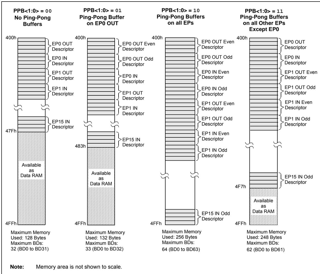
**TABLE 24-2: ASSIGNMENT OF BUFFER DESCRIPTORS FOR THE DIFFERENT BUFFERING MODES**
