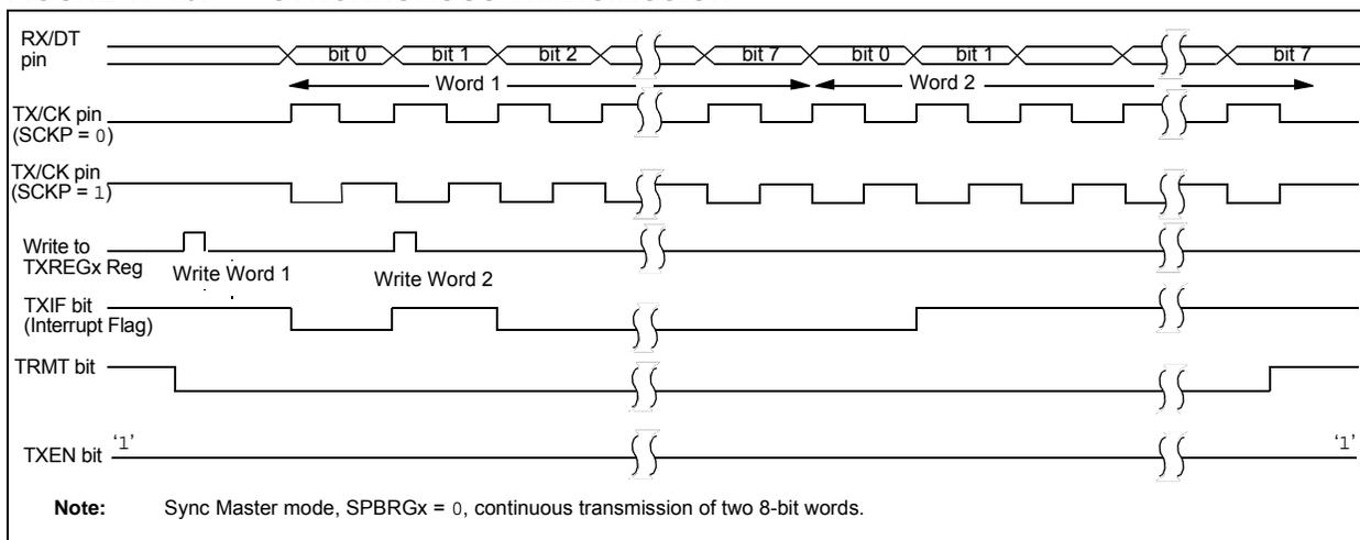
**FIGURE 17-11: SYNCHRONOUS TRANSMISSION (THROUGH TXEN)**
