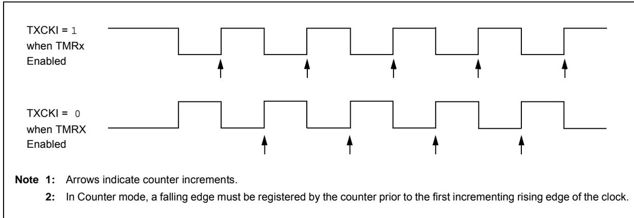
**FIGURE 13-4: TIMER1/3 GATE ENABLE MODE**
