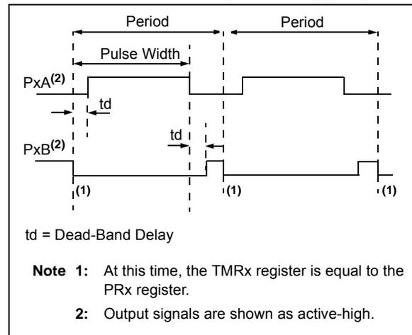
**FIGURE 15-17: EXAMPLE OF HALF-BRIDGE APPLICATIONS**
