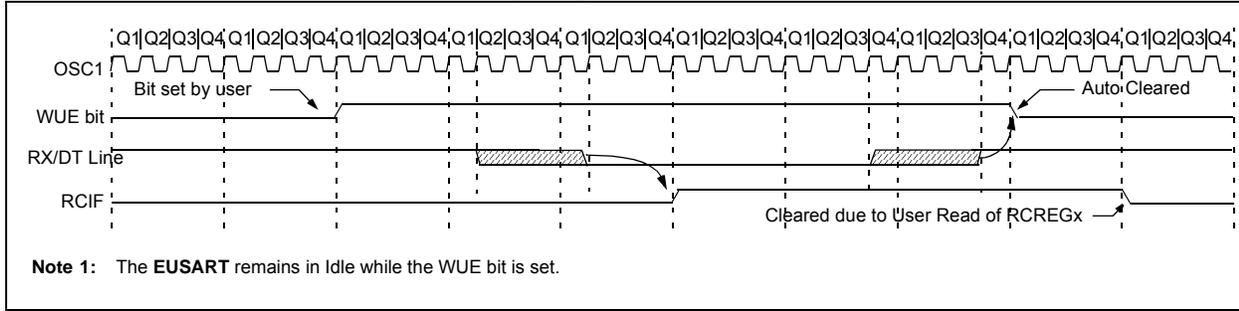
**FIGURE 17-8: AUTO-WAKE-UP BIT (WUE) TIMINGS DURING SLEEP**
