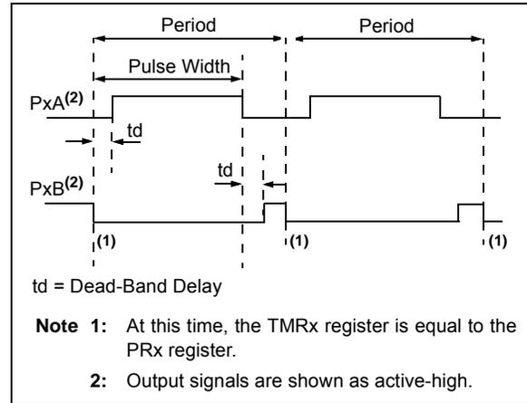
**FIGURE 15-9: EXAMPLE OF HALF-BRIDGE APPLICATIONS**
