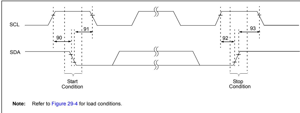
**TABLE 29-18: MASTER SSP I<sup>2</sup>C™ BUS START/STOP BITS REQUIREMENTS**
