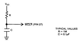
Master Clear may require up to a 75ms delay before activation after power is applied to the  $V_{DD}$  pin for a 1MHz crystal to start up. To achieve this an external RC configuration as shown can be used (assuming  $V_{DD}$  is applied as a step function). The RC oscillator option, shown above, should start up in less time.
