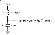
Master Clear requires >1.0ms delay before activation after power is applied to the  $V_{\rm DD}$  pin, for the oscillator to start up. To achieve this, an external RC configuration as shown can be used (assuming  $V_{\rm DD}$  is applied as a step function).
