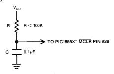
Master Clear requires 10ms delay (assuming a 4MHz crystal) before activation after power is applied to the  $V_{DD}$  pin, for the crystal to start up. To achieve this, an external RC configuration as shown can be used (assuming  $V_{DD}$  is applied as a step function).
