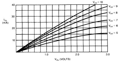
The Output Sink Current is dependent on the  $V_{\chi\chi}$  supply and the output load. This chart shows the typical curves used to express the output drive capability.
