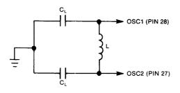
$$\label{eq:fosc} \begin{split} f_{\rm OSC} \approx & \frac{1}{2\pi \, \sqrt{L \, \left(C_L \, + C_{\rm INT}\right)}} \; , \\ & \text{where } C_{\rm INT} = 10 \text{pF}. \end{split}$$
