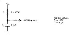
The  $\overline{MCLR}$  signal only needs to be active low for a minimum of 1 complete instruction cycle, but this assumes power is already applied, and the oscillator is running. For initial start-up at least a 10ms delay after  $V_{DD}{\geqslant}4.5V$  should be typically allowed on  $\overline{MCLR}$  for a 4 MHz crystal to start up.
