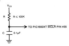
Master Clear requires 10ms delay (assuming a 4MHz crystal) before activation after power is applied to the  $V_{DD}$  pin, for the crystal to start up. To achieve this, an external RC configuration as shown can be used (assuming  $V_{DD}$  is applied as a step function).
