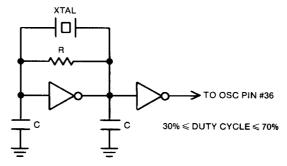
The buffer must be capable of driving  $120\Omega$ , min.  $(800\Omega$ , typ.) to 2.0V. However, it is recommended that the pull-down transistor on the OSC pin be removed (an option) if OSC is to be driven externally.
