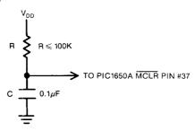
Master Clear requires >1.0ms delay before activation after power is applied to the  $V_{\mathrm{DD}}$  pin, for the oscillator to start up. To achieve this, an external RC configuration as shown can be used (assuming  $V_{\mathrm{DD}}$  is applied as a step function).
