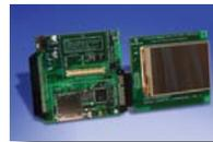
This kit provides a cost-effective method for evaluating and developing graphics display applications for 16- and 32-bit microcontrollers. It includes a Graphics LCD Controller PICtail Plus SSD1926 board (AC164127-5) and a Graphics Display Truly 3.2" 240 x 320 board (AC164127-4). The kit is compatible with the Explorer 16 development board (DM240001) or one of the PIC32 starter boards (DM320001, DM320003).
