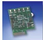
This daughter board demonstrates the MCP4725 (12-bit DAC with non-volatile memory) features using the Explorer 16 development board and the PICkit Serial Analyzer.
