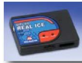
MPLAB REAL ICE In-Circuit Emulator System is Microchip's next generation high speed emulator for Microchip Flash DSC and MCU devices. It debugs and programs PIC and dsPIC Flash microcontrollers with
