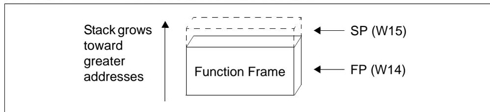
The C run-time startup modules (`crt0.o` and `crt1.o` in `libpic30.a`) initialize the Stack Pointer W15 to point to the bottom of the stack and initialize the Stack Pointer Limit register to point to the top of the stack. The stack grows up and if it should grow beyond the value in the Stack Pointer Limit register, then a stack error trap will be taken. The user may initialize the Stack Pointer Limit register to further restrict stack growth.
