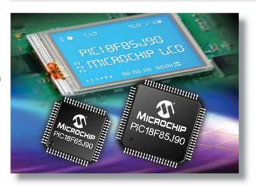
Microchip supports several families of microcontrollers with on-chip LCD driver control including the Mid-Range PIC16 and High Performance PIC18 families. The breadth of LCD segment drivers, package sizes and integrated features for embedded control application gives the designer flexibility to create different solutions based on the demand of varying market segments all from a single design.
