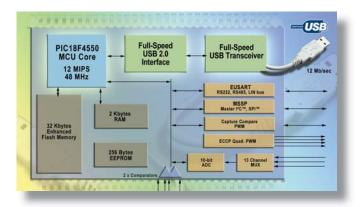
Microchip offers USB solutions capable of full-speed USB operation (up to 12 Mbits/s) in a new PIC18F family of devices, as well as low-speed operation (1 Mbits/s) in PIC16C devices.
