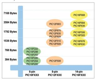
Microchip offers the most complete family of low pin count Flash microcontrollers available. These devices range from easy-to-use 6-pin microcontrollers, which can replace discrete logic functions, to 20-pin microcontrollers with advanced analog and communications peripherals that can serve as the central processor in an application.
