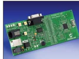
The PICDEM FS-USB (DM163025) is a demonstration and evaluation board for the PIC18F4550 family of Flash microcontrollers with full-speed USB 2.0 interface. The board contains a PIC18F4550 microcontroller in a 44-pin TQFP package, representing the superset of the entire family of devices.
