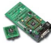
The PICDEM™ HPC Explorer Board (DM183022) is a low-cost tool ideally suited for evaluating the performance of Microchip's high memory and high pin count PIC18F 8-bit microcontrollers. This board can be used to demonstrate many PIC18F devices, including PIC18F8722 and PIC18F87J10 families.
