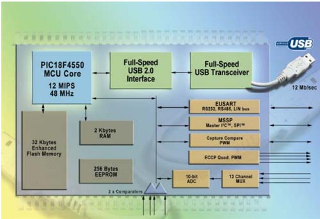
Microchip offers USB solutions capable of full-speed USB operation (up to 12 Mbits/s) in a new PIC18F family of devices, as well as low-speed operation (1 Mbits/s) in PIC16C devices.
