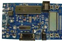
The PICDEM™ Low Power Solutions Demonstration Board (DM163026) gives designers a convenient and fun way to explore the nanoWatt technology features of PIC microcontrollers within a functional ultrasonic range-finder application using the PIC18F4620.
