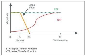
**Modulator Order** – The modulator order refers to the complexity of the delta-sigma architecture and amount of feedback in the analog design of the ADC. Higher order modulators can yield greater dynamic range due to a better noise-shaping. Noise falls by 3(2L-1) dB for each doubling of the over-sampling rate, where L is equivalent to the modulator order.
