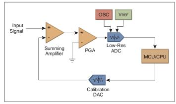
The design tip is to use a higher resolution ADC to your advantage when dealing with systems such as this. The entire signal conditioning circuitry can be eliminated if a higher resolution ADC such as the MCP355X is used:
