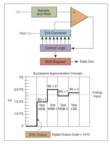
When designing a system with a SAR converter, the following specifications and terms should be understood:
