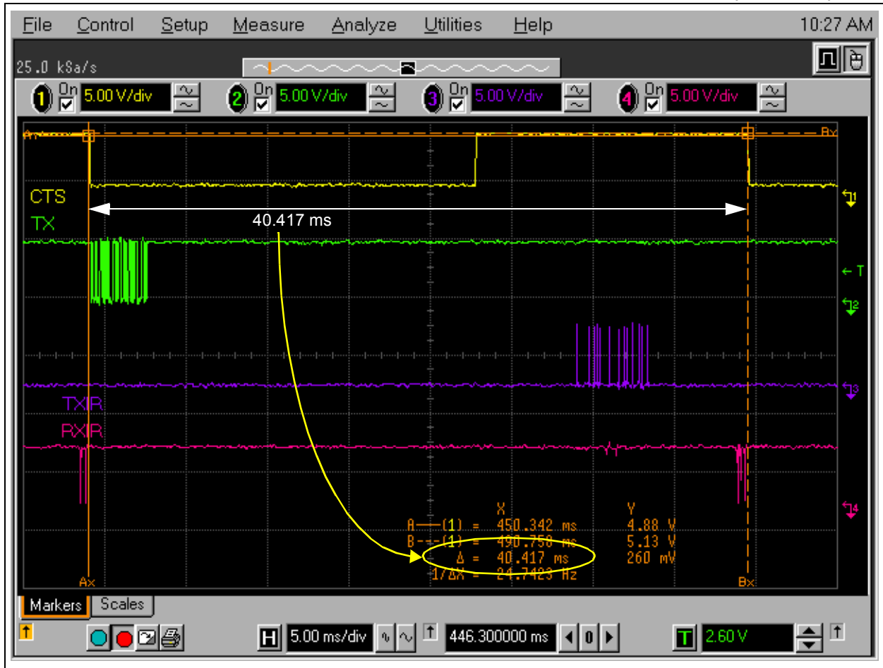
FIGURE 5: CTS TO CTS WHEN MCP215X RECEIVE BUFFER IS NOT FILLED (40 BYTES)
