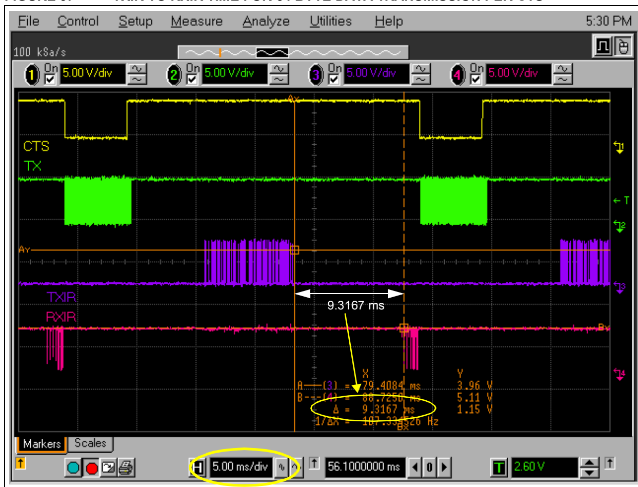
FIGURE 9: TXIR TO RXIR TIME FOR 64 BYTE DATA TRANSMISSION PER CTS
