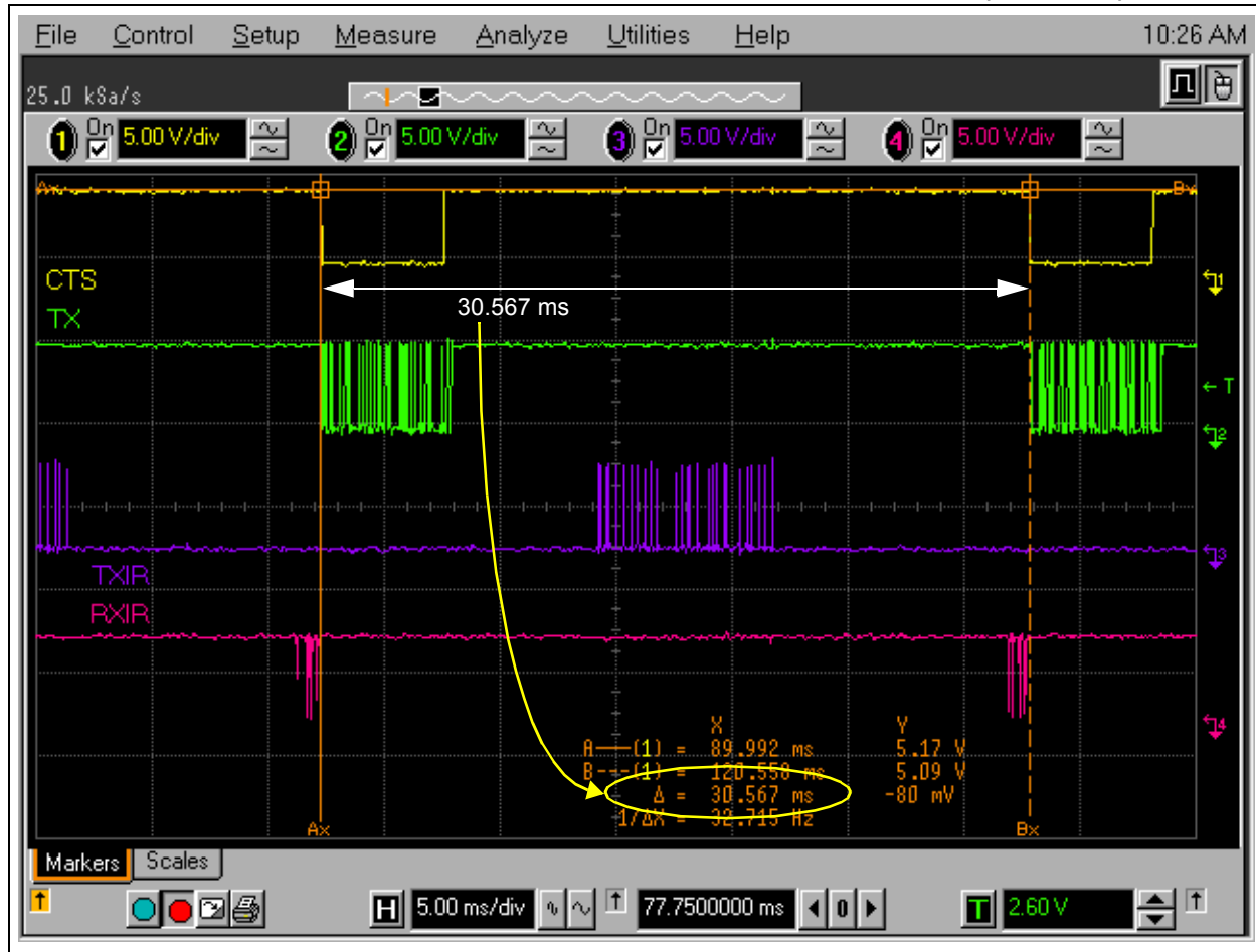
FIGURE 6: CTS TO CTS WHEN MCP215X RECEIVE BUFFER IS FILLED (64 BYTES)
