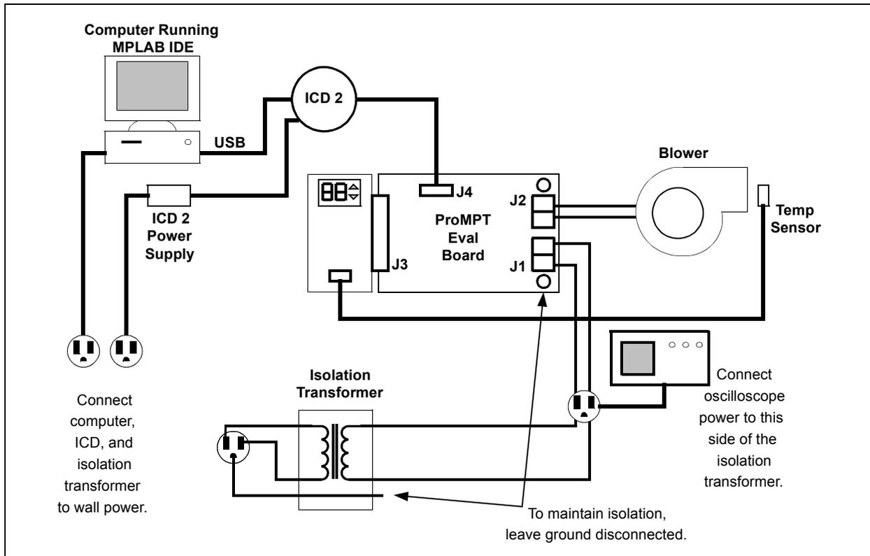
**Note:** Even with the isolation transformer, the ProMPT drive cannot be operated with MPLAB ICD 2 connected. To operate the motor (motor frequency greater than zero), MPLAB ICD 2 must always be disconnected.
