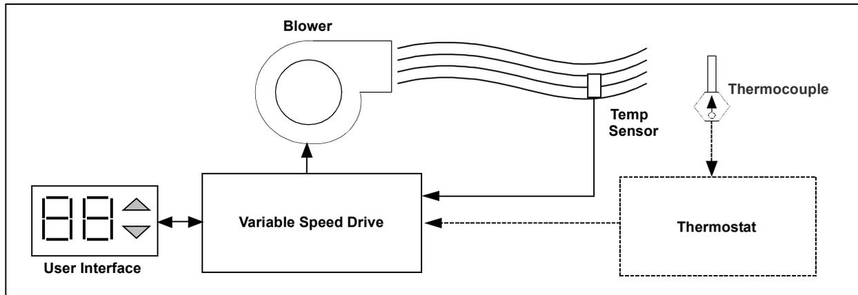
**FIGURE 2: VARIABLE SPEED RESPONSE**
