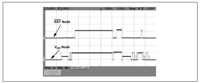
FIGURE 3: Successful programming waveform.
