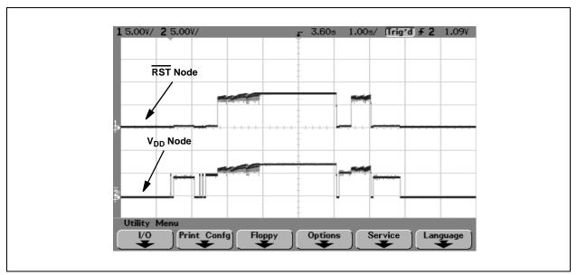
FIGURE 5: Failed verify programming waveform.
