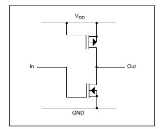
FIGURE 1: MCP120 output stage simplified.
