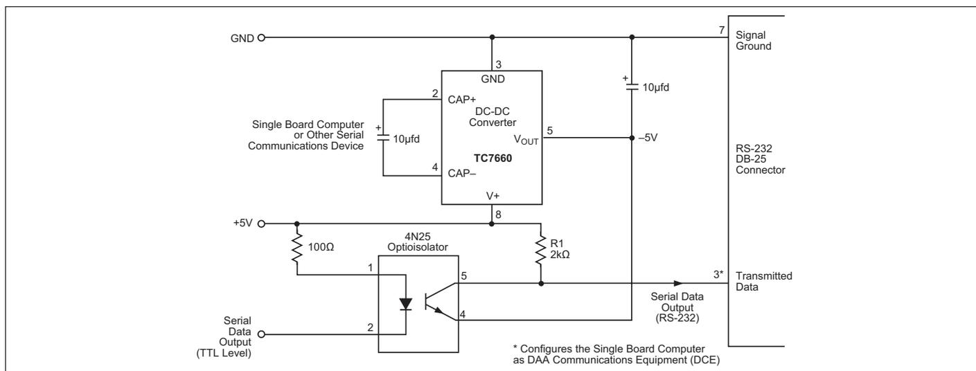
FIGURE 1: This low cost circuit converts TTL-level signals to an RS-232 level without the expense of a negative power supply. The TC7660's -5V output permits the optoisolator to swing to RS-232 levels at up to 9600 baud.
