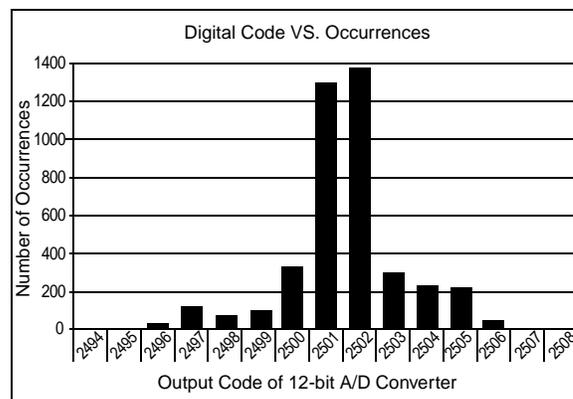
**FIGURE 6:** This is a histogram of 4096 samples from the output of the A/D Converter on the PCB that has a ground plane as shown in the PCB layout in Figure 5. Note that the power traces are made considerably wider than the signal traces in order to reduce power supply trace inductance. This circuit has all by-pass capacitors installed.
