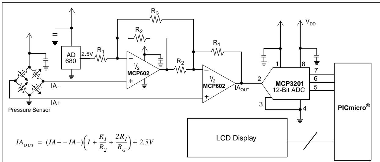
**FIGURE 1:** This is a pressure sensor application where the differential signal from the sensor is gained by an instrumentation amplifier and digitized with a 12-bit A/D Converter, MCP3201. The results of the conversion is displayed on the LCD display.
