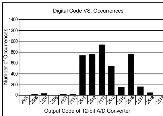
**FIGURE 8:** This a histogram of 4096 samples from the output of the A/D Converter on the PCB that has a ground plane as shown in the PCB layout in Figure 3. With this circuit implementation, all by-pass capacitors have been removed.
