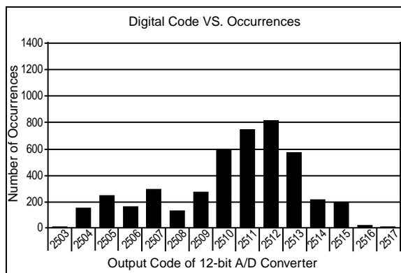
**FIGURE 4:** This is a histogram of 4096 samples from the output of the A/D Converter from a PCB that does not have a ground or power plane as shown in the PCB layout in Figure 3. The by-pass capacitors are installed.
