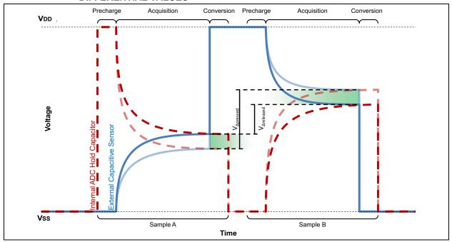
Finally, calculate the total CVD signal by subtracting the unpressed differential from the pressed differential. Equation 5 is the amount of change in the sensor reading due to the finger being added to the circuit. This is the value we should design to maximize.
