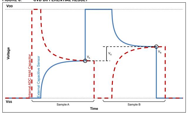
Note: In software, it's recommended to offset the value of V<sub>B</sub> by 2<sup>N</sup> (where N is the number of bits in the ADC) to further ensure a negative result is never achieved. For these calculations, this offset has been ignored to simplify the math.
