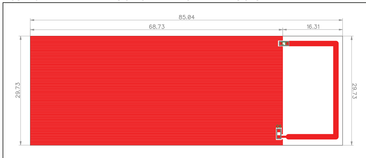
FIGURE 3: ANTENNA DESIGN. OVERALL BOARD DIMENSIONS
