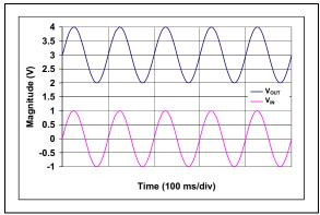
*FIGURE 29:* Op Amp Clamp Circuit Simulation Result.
