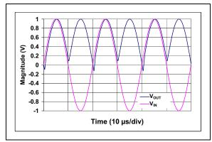
FIGURE 21: Circuit Behavior when Input Frequency = 100 kHz.
