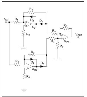
FIGURE 36: Three Stage Full-Wave Rectifier.
