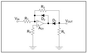
FIGURE 15: Negative Half-Wave Rectifier.
