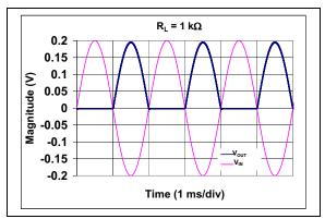
**FIGURE 13:** Improved Half-Wave Rectifier with  $R_L = 1 \ K\Omega$ .
