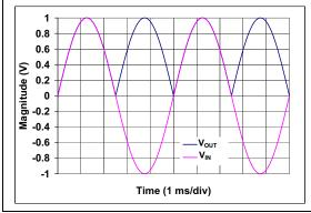
FIGURE 20: Full-Wave Rectifier Circuit Simulation.
