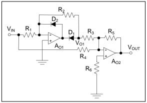
FIGURE 19: Two Stage Op Amp Full-Wave Rectifier Circuit.
