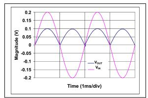
**FIGURE 18:** Full-Wave Rectifier Circuit Simulation with the Recommended Values of the Resistors.
