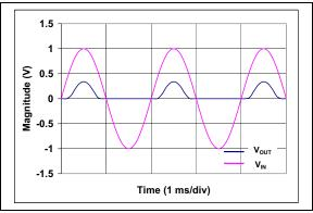
FIGURE 5: Positive Half-Wave Rectifier Sample.
