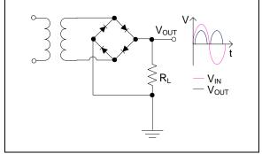
FIGURE 3: Full-Wave Rectifier.
