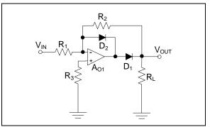
FIGURE 12: Have-Wave Rectifier Circuit Improvement.
