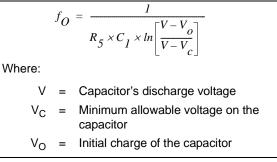
The response time describes how quickly  $C_1$  can respond to the decreases in the magnitude of the input signal. This can be computed from the basic discharge equation. However, if we assume that the capacitor is charged to peak and discharges towards an eventual value of 0, we can use the simplified form (Equation 14).
