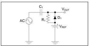
FIGURE 26: Basic Diode Negative Clamp.
