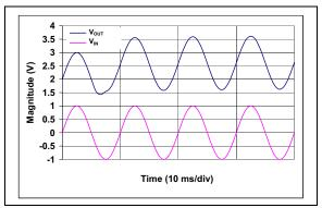
FIGURE 27: Basic Diode Clamp – Circuit Simulation.
