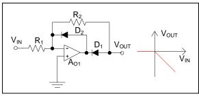
FIGURE 33: Negative Half-Wave Rectifier 2.
