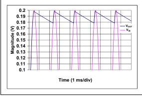
FIGURE 25: One Peak Detector Simulation Results.
