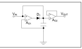
FIGURE 38: Peak Detector Rectifier 2.
