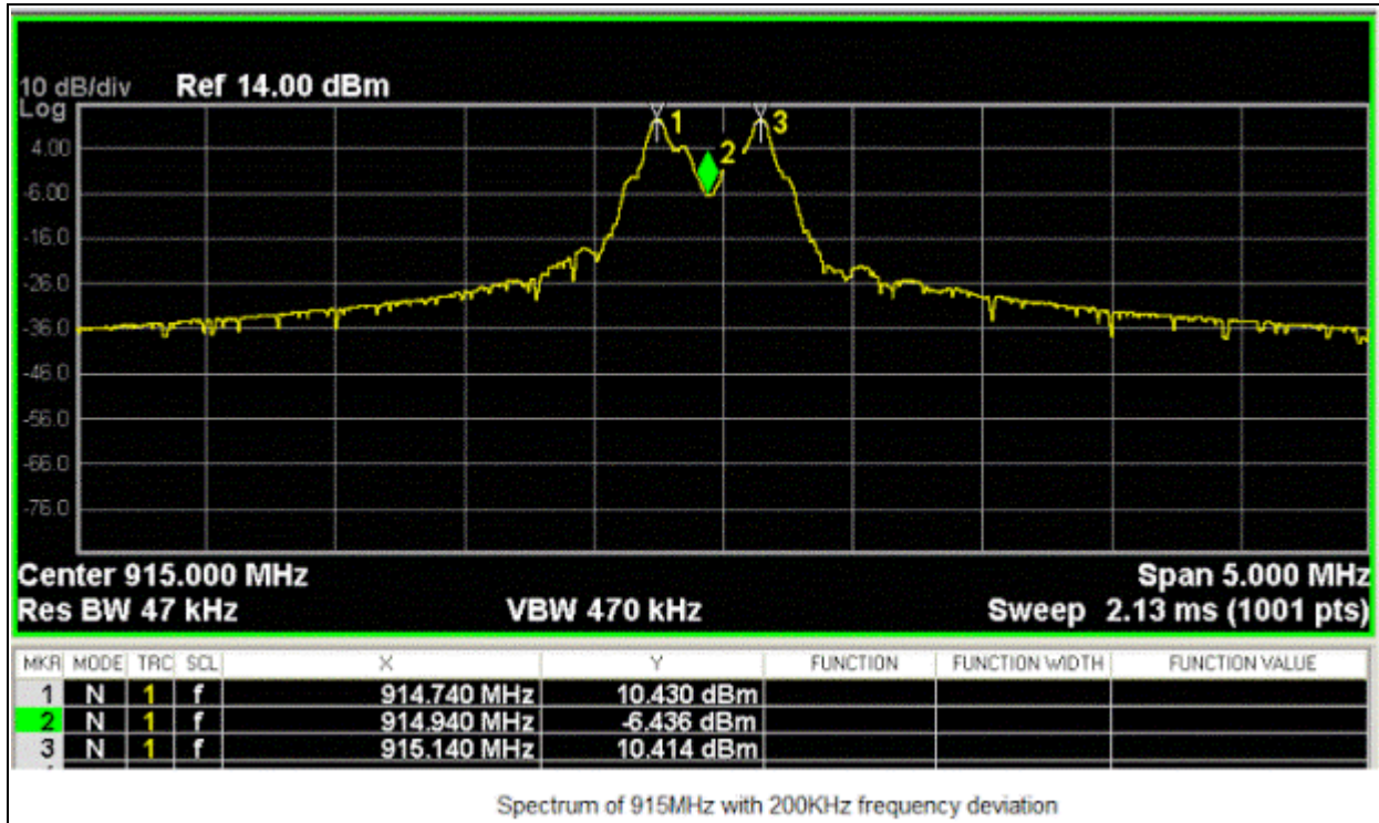
FIGURE 23: CAPTURING THE TRANSMISSION ON SPECTRUM ANALYZER
