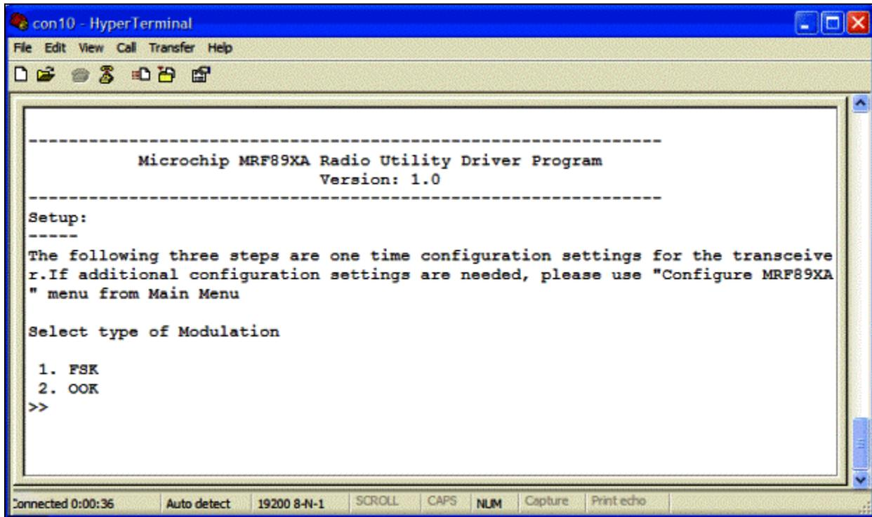
After powering the PIC18 Explorer or the Explorer 16 development boards with the MRF89XA daughter card, the user must configure the default mode of operation by following these setup procedure.
