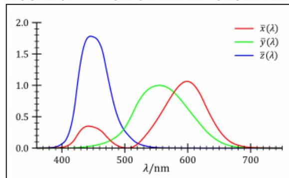
The TCS3414CS RGB sensor contains filters that reproduce this spectral response, enabling it to closely match the response of the human eye. Additionally, the sensor utilizes an infrared (IR) filter that blocks IR energy that would otherwise saturate the sensor. Figure 4 shows the spectral response of the sensor due to these filters.
