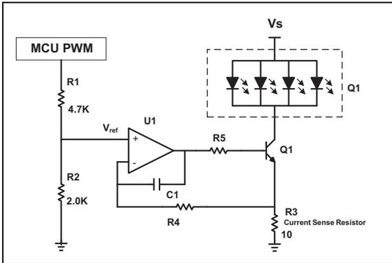
Current is controlled by adjusting  $V_{REFOUT}$  and the value of  $R3$  to produce the current output desired by using Equation 1.
