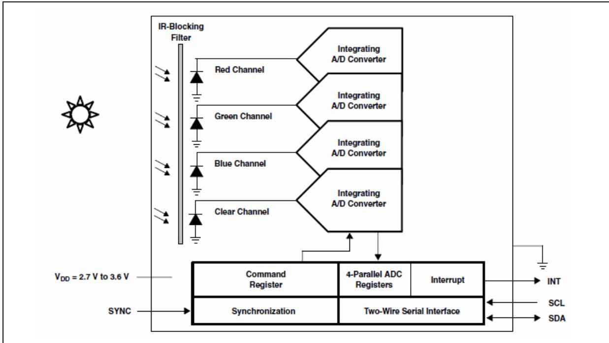
The TCS3414CS uses a light to frequency converter to measure the intensity of incident light. The wavelength of the light is filtered by red, green, blue and clear filters. An infrared filter eliminates contributions from wavelengths above 680 nm over the entire spectrum. These RGB filters provide a means to separate the primary wavelengths of the visible spectrum that the human eye perceives as color. The clear filter provides a measure of the intensity of light over the visible spectrum.
