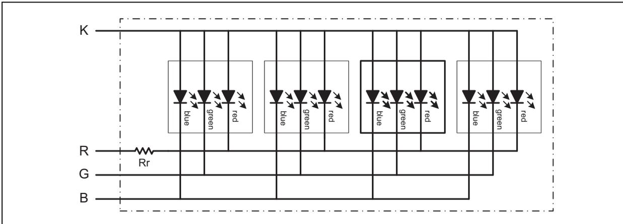
**Note:** Driving the LED strings at 80 mA results in thermal rise on the LED PCB that cannot be easily dissipated. This rise in thermal conditions causes the LED outputs to drift when an LED string was driven near 100% duty cycle. In order to eliminate the output drift in the LEDs, the driver circuit must be reduced to drive at 55 mA. This eliminates the thermal issue and allows a stable control system.
