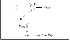
**FIGURE 10:** Application to Inverting Bias Current Error Calculations.
