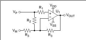
FIGURE A-1: Offset Test Circuit.
