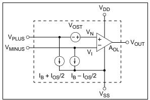
**FIGURE 3:** Equivalent DC Model for Traditional Op Amps.
