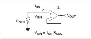
**FIGURE 6:** Application to Non-inverting Bias Current Error Calculations.
