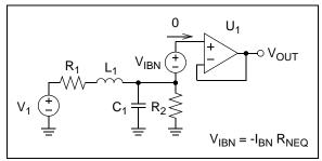
**FIGURE 7:** Application to Non-inverting Bias Current Error Calculations.
