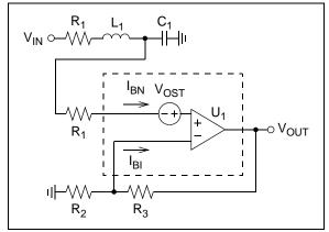
FIGURE 14: Non-inverting Gain Amplifier.
