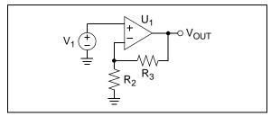
FIGURE 8: Non-inverting Gain Circuit.
