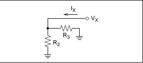
FIGURE 9: Equivalent DC Circuit for the Inverting Input.
