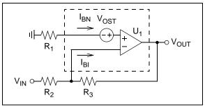
FIGURE 15: Inverting Gain Amplifier.
