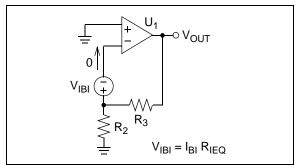
**FIGURE 11:** Application to Inverting Bias Current Error Calculations.
