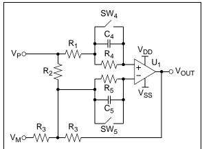
FIGURE A-2: Offset Test Circuit with Bias Current Capabilities.
