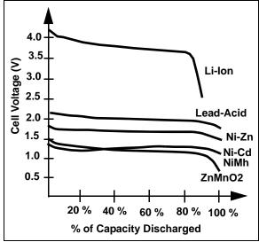
FIGURE 1: Battery Discharge Characteristics.
