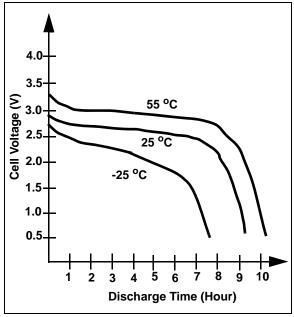
FIGURE 2: LI-lon Battery Discharge Characteristics vs. Temperature.
