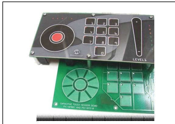
The demo boards shown in Figure 5 are more easily constructed compared to adhesively attaching the covering plate to the PCB, especially with the paper in between. Some interesting parts are used in the demo, such as backward facing surface mount LEDs to shine through holes cut in the PCB. The bill of materials is listed in **Appendix A: “Multibutton Capacitive Demo Board”** for reference.
