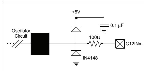
If the voltage rises above VDD + 0.7 volts, the top diode turns on and current flows into the capacitor. If the voltage goes below GND - 0.7 volts, the bottom diode turns on and current flows from the capacitor into the circuit. A nearly identical system is inside the microcontroller's I/O pin. The 100 ohm resistor ensures that the external diodes trigger first. This circuit has been tested to have minimal interference with capacitive sensing operations.
