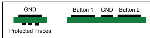
For applications with a lot of electromagnetic interference, shielding the traces leading to the pads will improve immunity. Obviously, the button interface may not be completely surrounded by ground, but if the inside of the panel can be shielded, it will help protect against EMI related problems.
