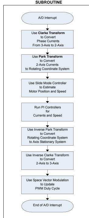
Figure 28 illustrates the process of using the Slide-Mode Controller to estimate the position and speed of the motor.
