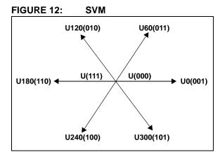
The process of SVM allows the representation of any resultant vector by the sum of the components of the two adjacent vectors. In Figure 13, UOUT is the desired resultant. It lies in the sector between U60 and U0. If during a given PWM period T, U0 is output for T1/T and U60 is output for T2/T, the average for the period will be UOUT.
