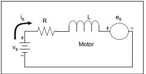
From the motor model, the input voltage can be obtained by Equation 1.
