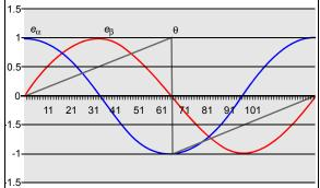
The plot shows a trigonometric function relating the vector components of the back-EMF ( $e_{\alpha}$  and  $e_{\beta}$ ) and rotor angle ( $\theta$ ). The arctangent is computed on the back-EMF vector components to calculate Theta. Equation 5 illustrates how the function is implemented in software:
