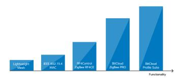
The Lightweight Mesh software stack is designed to work with all Atmel IEEE 802.15.4 transceivers and SoCs. Currently the stack works with Atmel AVR<sup>®</sup> microcontrollers (MCUs), but given its extreme portability and low resource requirements, it can be run on almost any Atmel MCU.
