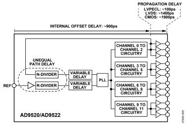
Figure 6. AD9520/AD9522 Internal Zero-Delay Timing Offset Errors
