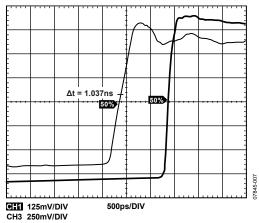
Figure 7. Internal Zero-Delay Intrinsic Offset Timing Error (AD9520)
