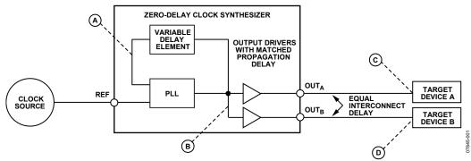
Figure 1. Generic Zero-Delay Synthesizer
