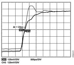
Figure 11. External Zero-Delay Adjusted Offset Timing (AD9520)
