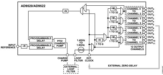
Figure 5. AD9520/AD9522 Functional Block Diagram
