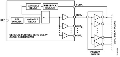
Figure 4. External Zero-Delay Architecture Rev. 0 | Page 3 of 8
