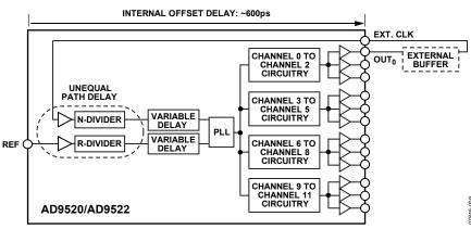
Figure 9. AD9520/AD9522 External Zero-Delay Timing Offset Error
