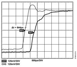
Figure 10. External Zero-Delay Inherent Offset Timing Error (AD9520)
