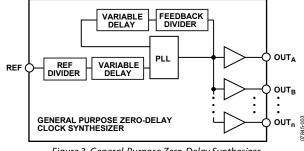
Figure 3. General-Purpose Zero-Delay Synthesizer
