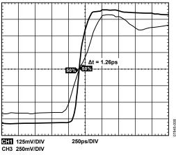
Figure 8. Internal Zero-Delay Adjusted Offset Timing (AD9520)
