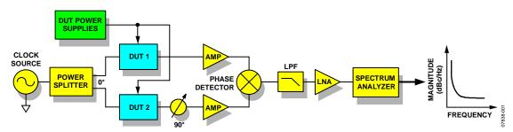
Figure 1. Residual Phase Noise Measurement Setup
