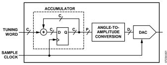
Figure 1. Typical Accumulator-Based DDS Architecture
