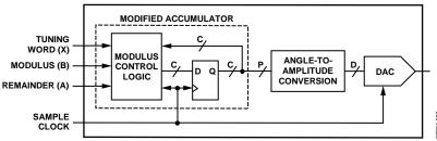
Figure 2. Programmable Modulus DDS Architecture
