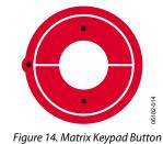
When the user activates any key in the keypad, status bits in the status registers are set. The host can read back data from the AD7142/AD7143 to determine the set status bits. Status bits for each column, and for each row, are used to determine which key is pressed. The decoding is the same as that required for conventional mechanical matrix keypads. The active key is at the location where both its row and column status bits are set.
