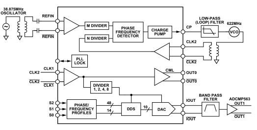
Figure 2. AD9540 Configured for Dual Clock Generation
