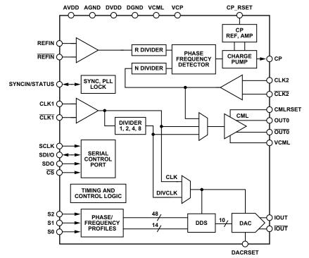
Figure 1. AD9540 Block Diagram
