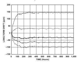
Figure 1. Typical Long-Term Drift Over 1,000 Hours
