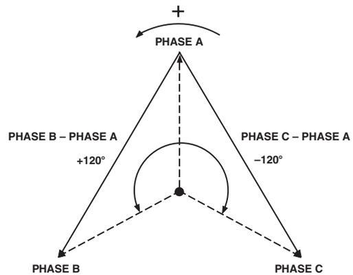
Figure 6. 3-Phase 3-Wire Delta Phasor Diagram
