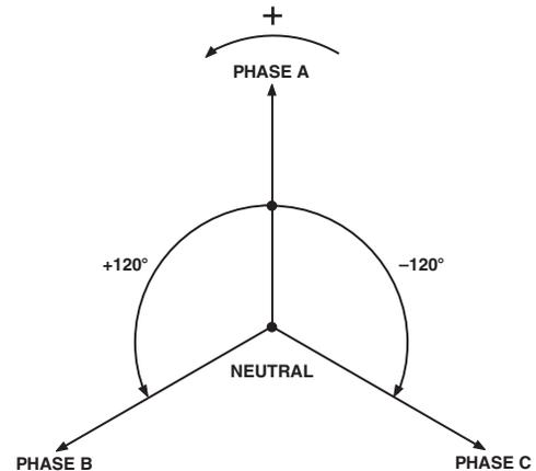
Figure 2. 3-Phase 4-Wire Wye Phasor Diagram
