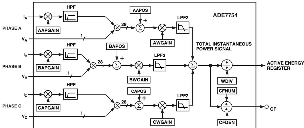
Figure 20. Total Active Energy Calculation
