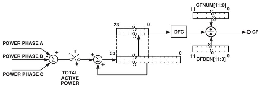
Figure 9. Energy-to-Frequency Conversion
