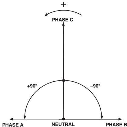
Figure 4. 3-Phase 4-Wire Delta Phasor Diagram
