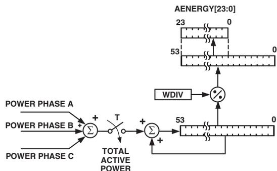
Figure 8. Active Energy Accumulation
