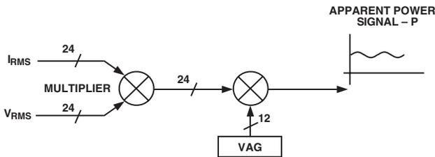
Figure 15. Apparent Power Signal Processing
