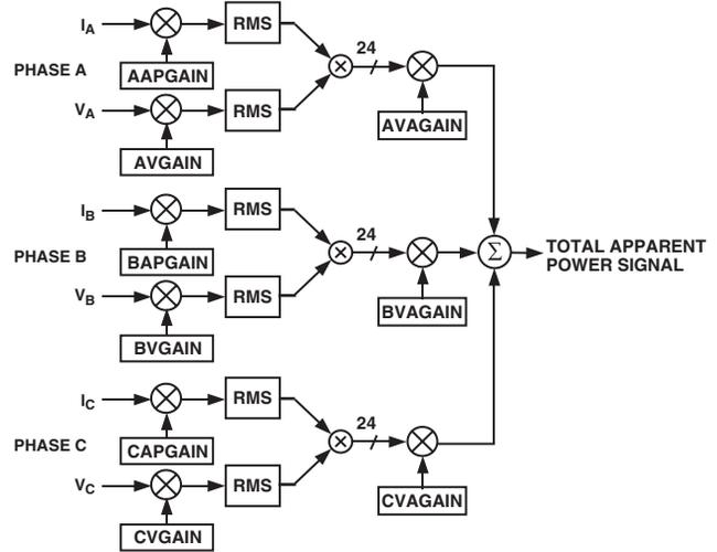
Figure 26. Total Apparent Energy Application
