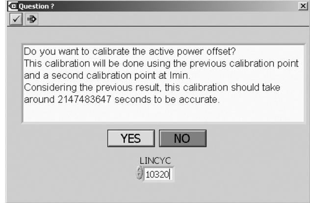
Figure 23. Change LINCYC Register for Offset Calibration
