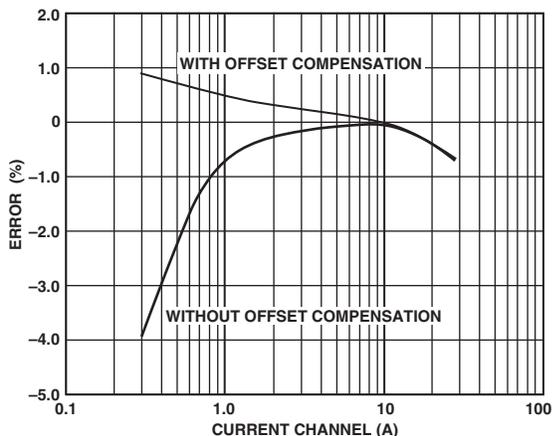
Figure 25. Current RMS Linearity Errors
