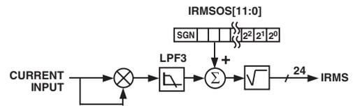
Figure 12. ADE7754 Current RMS Signal Processing
