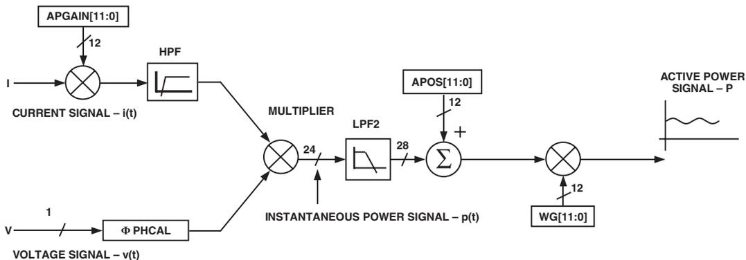
Figure 7. Active Power Signal Processing
