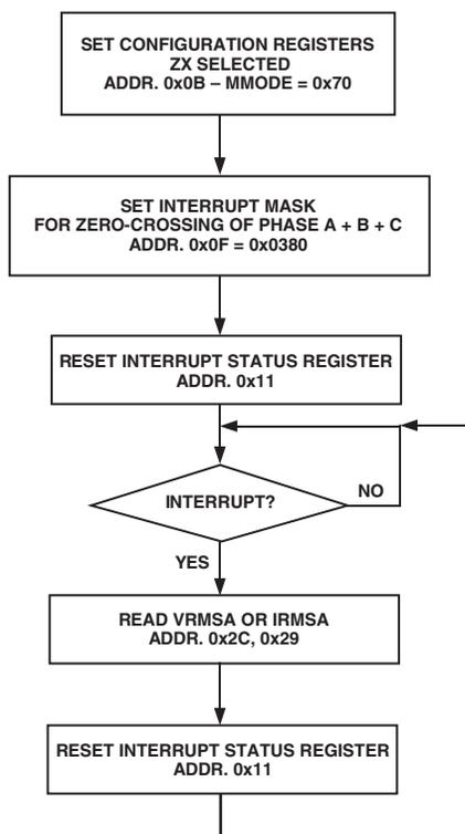
Figure 13. ADE7754 RMS Reading Setup for Phase A
