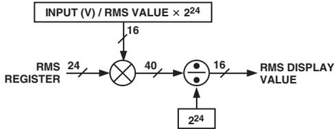
Figure 14. Conversion of the RMS Register in a Displayable Value
