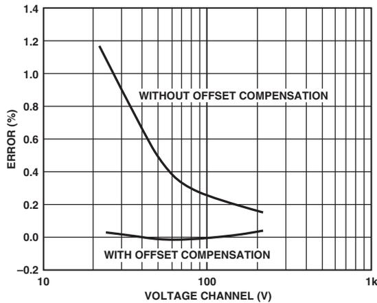
Figure 24. Voltage RMS Linearity Errors
