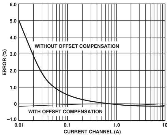
Figure 22. Active Energy Linearity Errors
