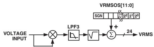
Figure 11. ADE7754 Voltage RMS Signal Processing
