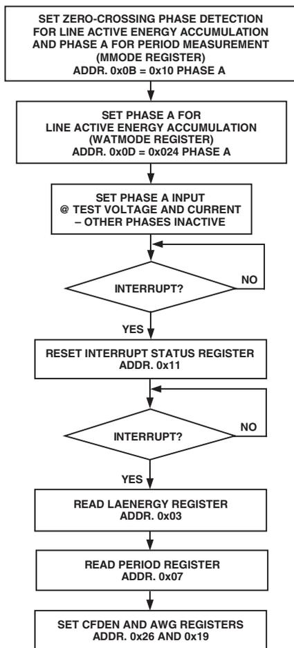
Figure 21. Active Energy Gain Calibration Procedure for Phase A
