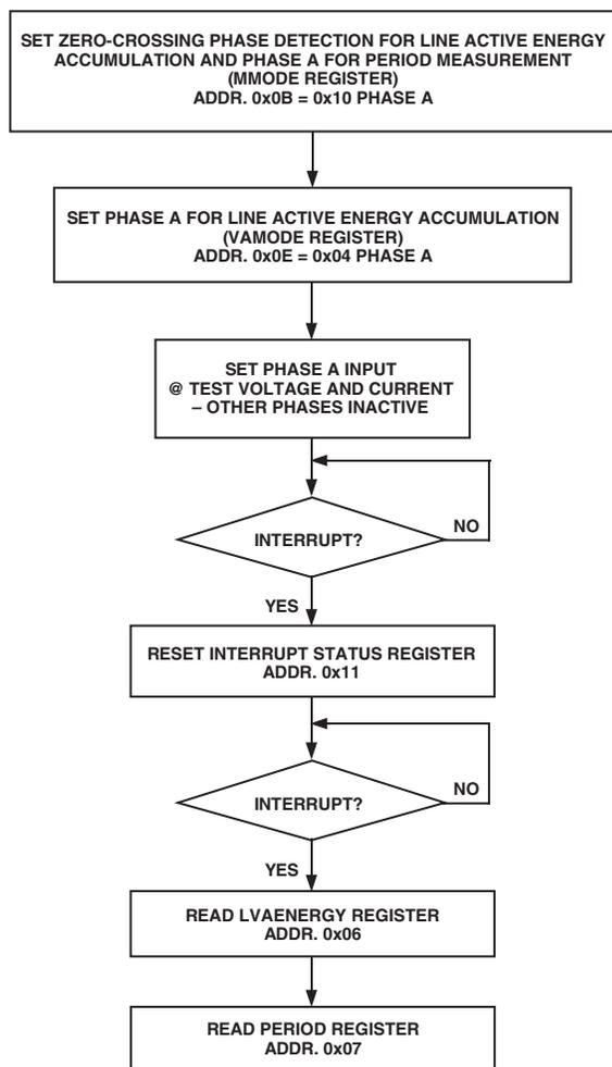
Figure 17. Apparent Energy Gain Calibration Procedure for Phase A
