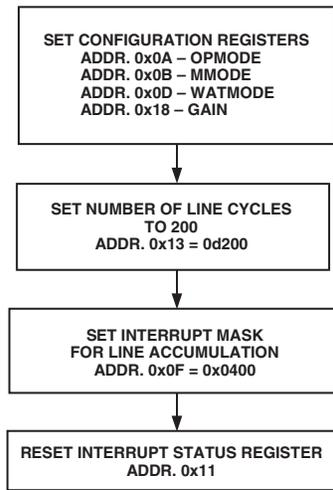
Figure 10. Line Accumulation Mode Setup
