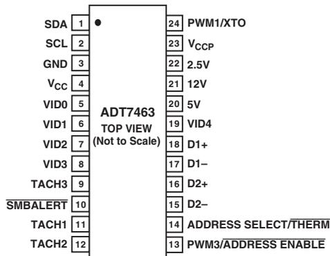
Figure 3. Pinout Option 2
