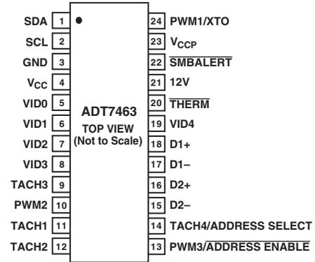
Figure 6. Pinout Option 5
