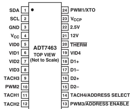
Figure 7. Pinout Option 6
