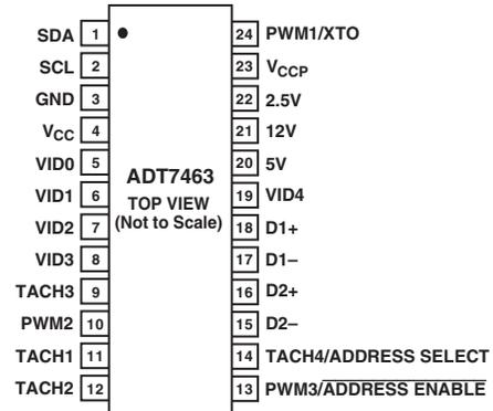
Figure 4. Pinout Option 3
