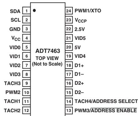
Figure 5. Pinout Option 4
