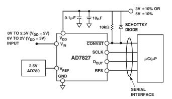
Figure 1. Typical Connection Diagram of the AD7827
