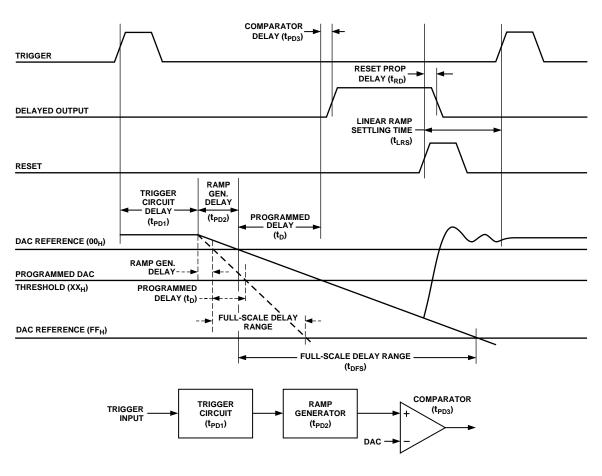
MINIMUM PROPAGATION DELAY =  $(t_{PD}) = (t_{PD1}) + (t_{PD2}) + (t_{PD3})$
