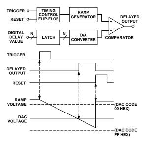
Figure 2. Delay Generator Block Diagram and Basic Timing
