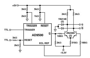
Figure 7. Interfacing the AD9500 with TTL
