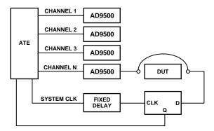
Figure 11. Automatic Calibration for ATE Deskew
