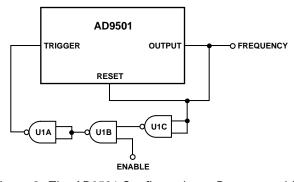
Figure 8. The AD9501 Configured as a Programmable Oscillator
