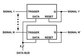
Figure 10. Multiple Signal Deskewing
