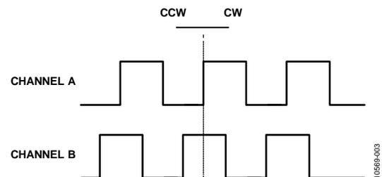
Figure 3. Mechanical Encoder Pulses
