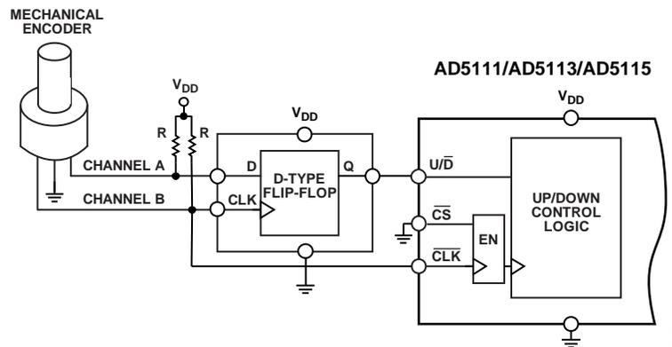
Figure 4. Circuit Diagram Connection
