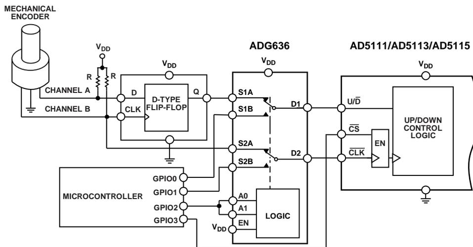
Figure 5. Hybrid Interface Connection
