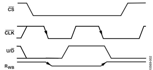
Figure 2. Up/Down Interface Operation
