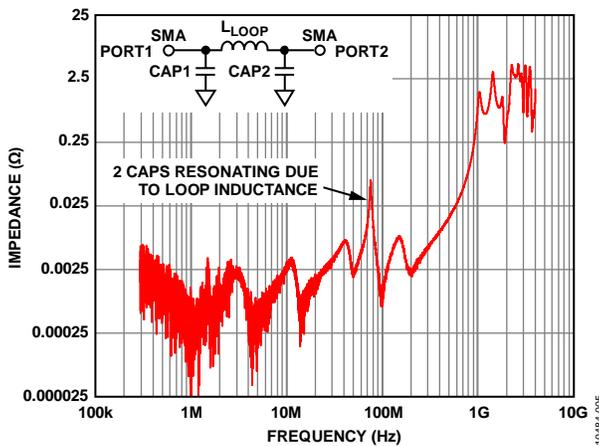
Figure 5. Resonating Capacitors
