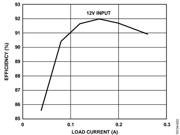
Figure 23. Converter Efficiency vs. Load Current
