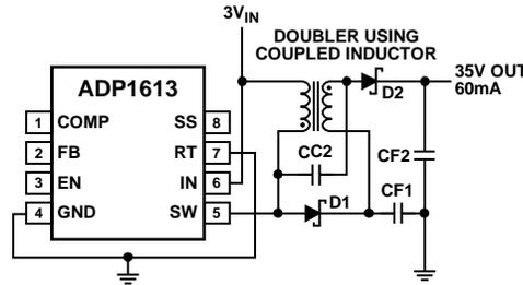
Figure 17. ADP1613 Standard Configuration
