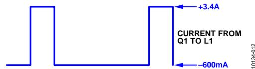
Figure 12. Current from Q1 to L1
