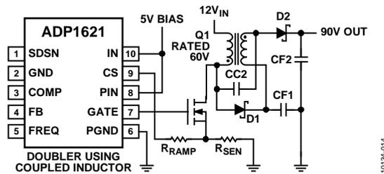
Figure 14. ADP1621 Standard Current Sense Resistor Configuration
