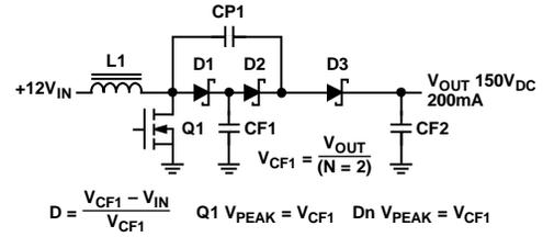
Figure 2. Charge Pump Multiplied Boost with Two Stages
