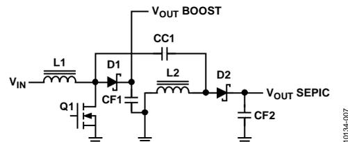
Figure 7. SEPIC Converter with Added Boost
