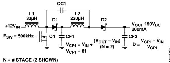
Figure 4. Two-Stage SEPIC Multiplied Boost Converter
