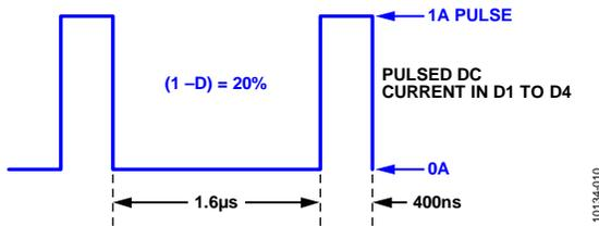
Figure 10. Current Waveform in Diode D1 through Diode D4
