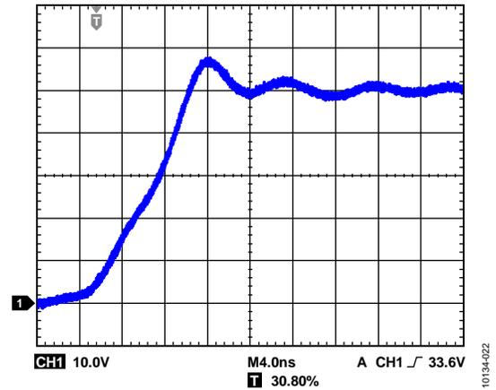
Figure 22. Switch Node Waveform During Full Load Operation, 4 ns per Division
