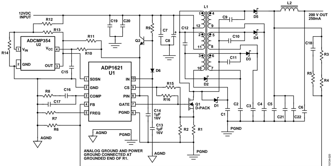
Figure 20. ADP1621 5x SEPIC Multiplied Boost (Tested Example)
