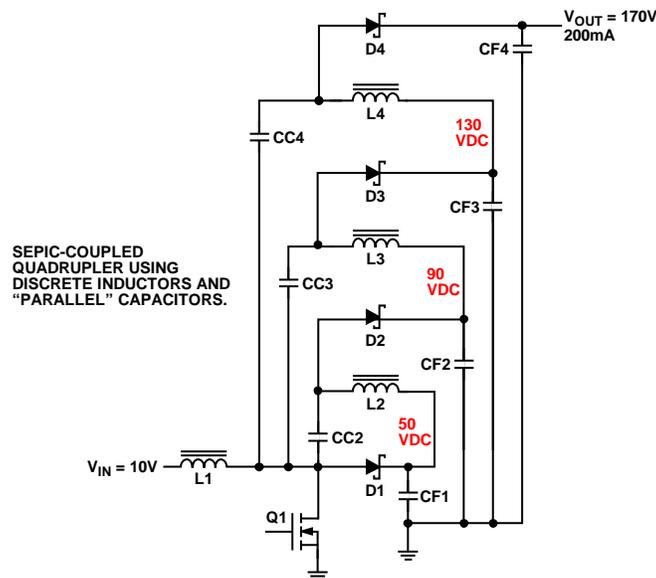
Figure 19. SEPIC-Coupled Quadrupler Using Discrete Inductors and Parallel Capacitors
