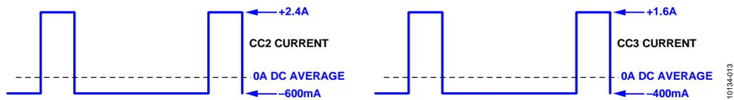
Figure 13. Current Waveforms Through CC2 and CC3, Respectively
