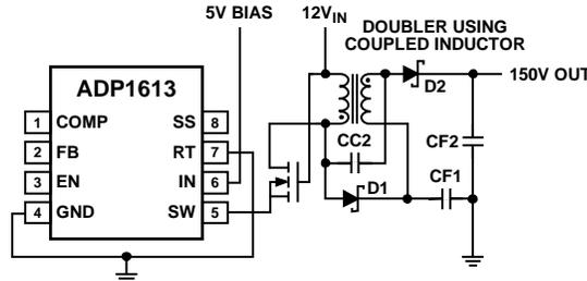
Figure 18. ADP1613 Cascode Configuration
