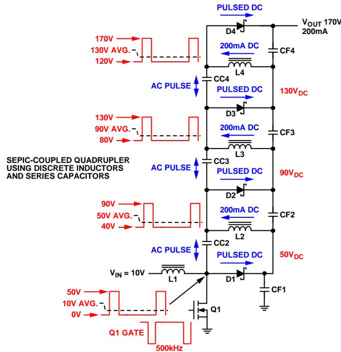
Figure 9. SEPIC-Coupled Quadrupler Using Discrete Inductors and Series Capacitors
