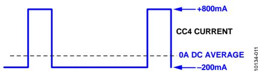
Figure 11. Current Waveform Through CC4
