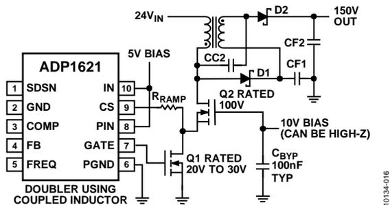
Figure 16. ADP1621 Cascode Configuration
