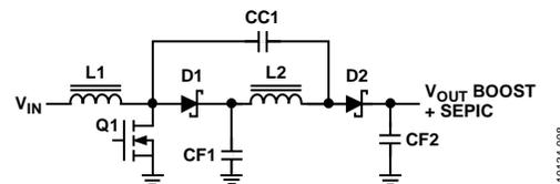
Figure 8. SEPIC Multiplied Boost Converter with  $N = 2$
