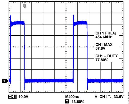
Figure 21. Switch Node Waveform During Full Load Operation, 400 ns per Division
