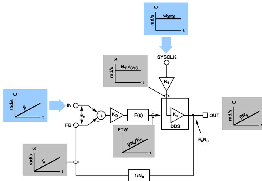
Figure 5. Frequency Ramp at the IN Terminal
