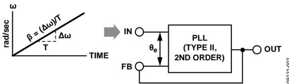
Figure 4. Linear Frequency Ramp Input
