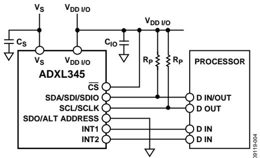
Figure 4. Recommended Connection for I<sup>2</sup>C Mode
