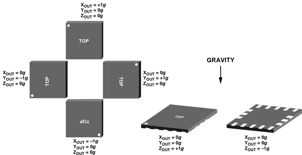
Figure 2. Output Response vs. Orientation to Gravity
