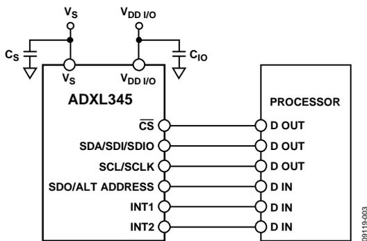
Figure 3. Recommended Connection for 4-Wire SPI Mode
