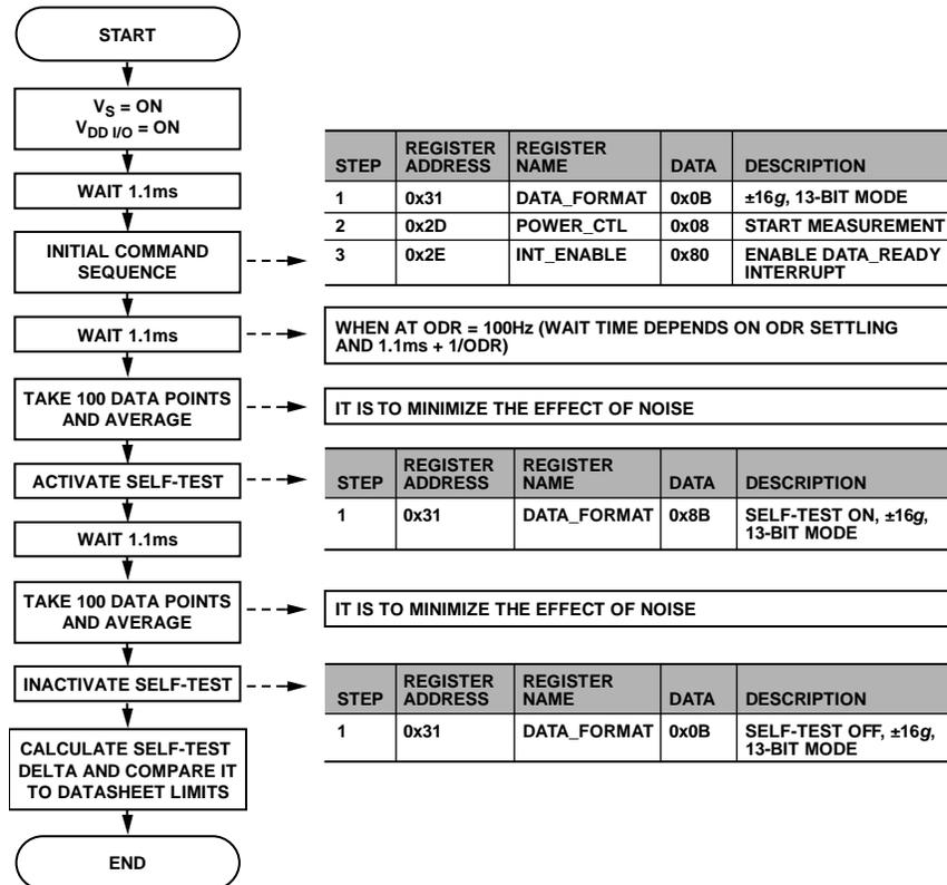
Figure 8. Self-Test Sequence
