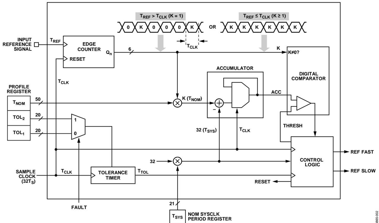
Figure 2. Reference Monitor Detailed Block Diagram
