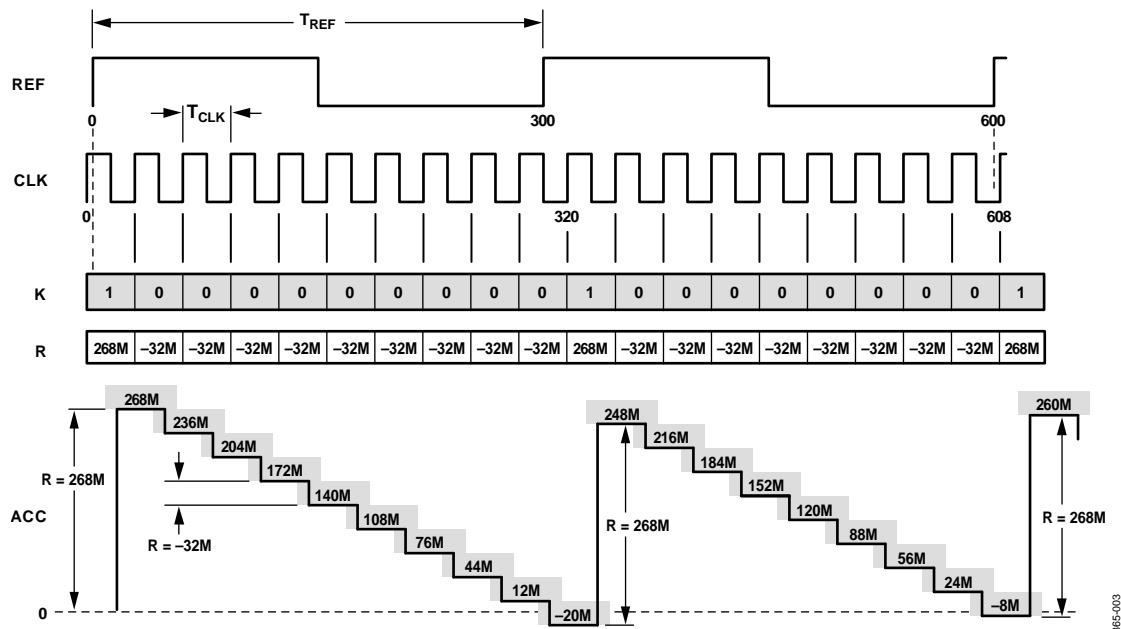
Figure 3. Accumulator Output Waveform for  $T_{REF} > T_{CLK}$
