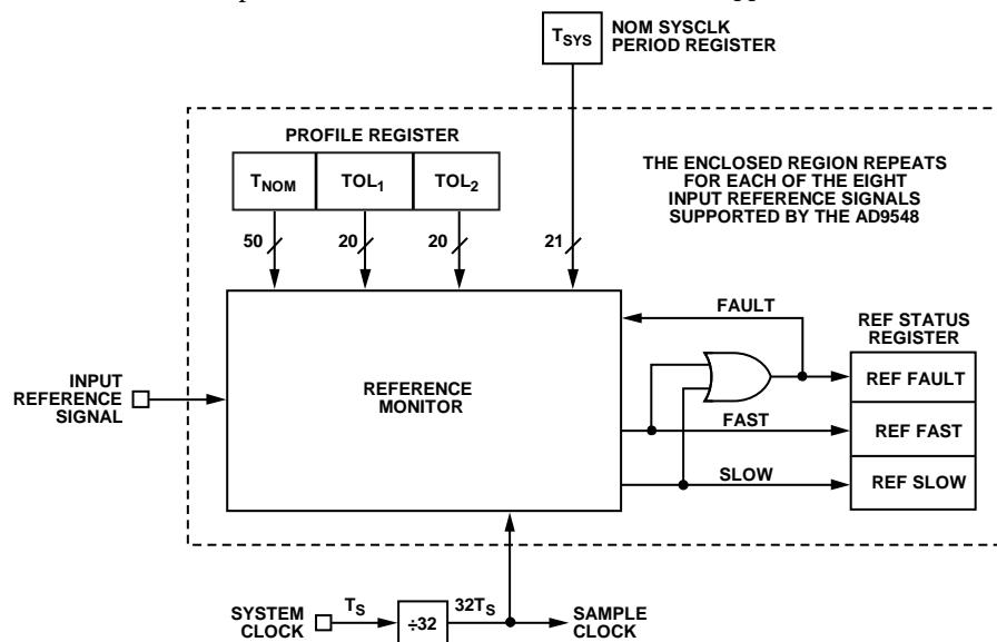
Figure 1. Reference Monitor and Supporting Elements
