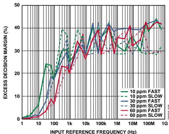
Figure 6. Excess Decision Margin for Tolerance = 10 ppm, 30 ppm, and 60 ppm
