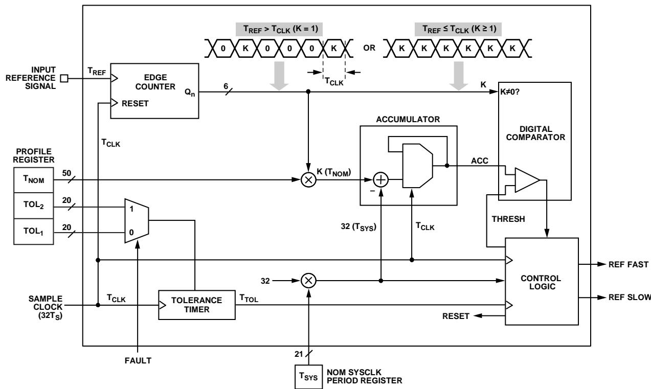
Figure 2. Reference Monitor Detailed Block Diagram
