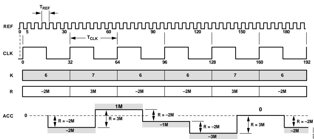
Figure 4. Accumulator Output Waveform for  $T_{REF} \leq T_{CLK}$
