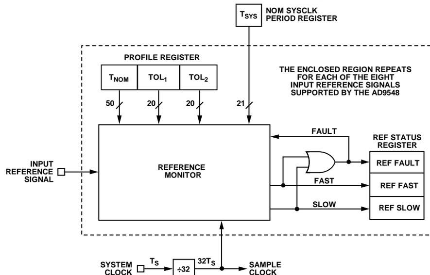
Figure 1. Reference Monitor and Supporting Elements
