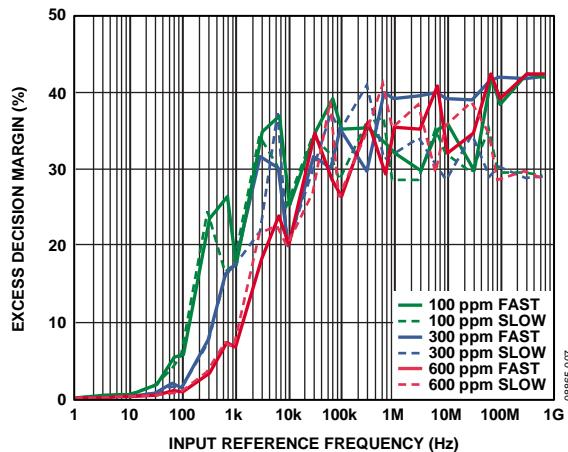
Figure 7. Excess Decision Margin for Tolerance = 100 ppm, 300 ppm, and 600 ppm
