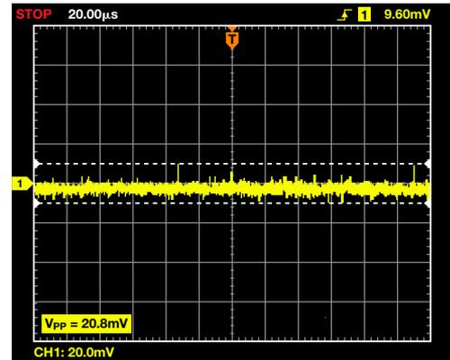
Figure 8. Ripple of 5-V supply on AV<sub>CC</sub> and DV<sub>CC</sub>.
