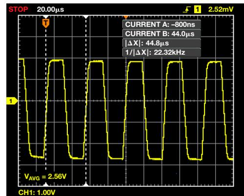
Figure 9. 22.32 kHz square waveform.
