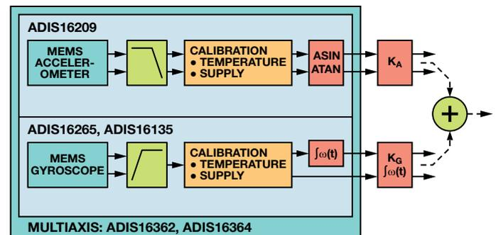
Figure 2. Combining single-axis sensor outputs.
