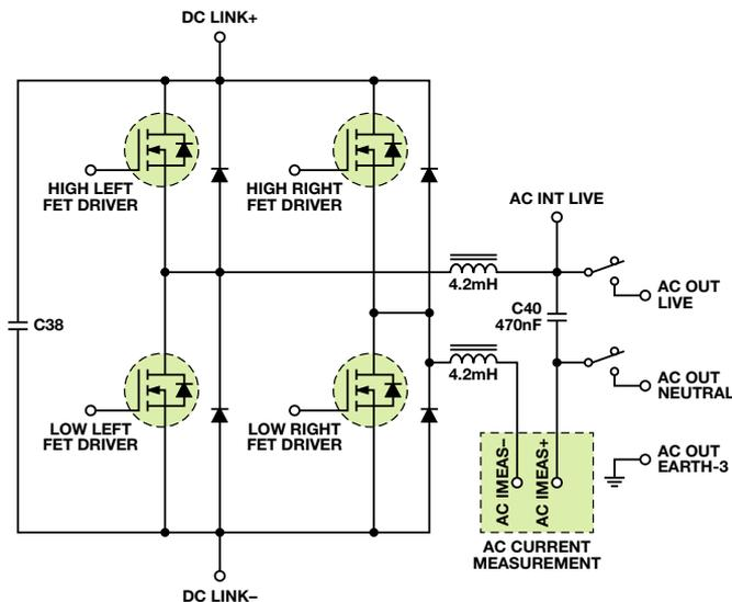
Figure 5. H-bridge circuit example for solar PV inverter.
