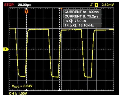
Figure 10. 13.16 kHz pulse waveform.
