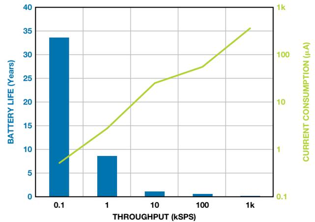
Figure 3. Battery life and current consumption vs. throughput for the AD7091R.
