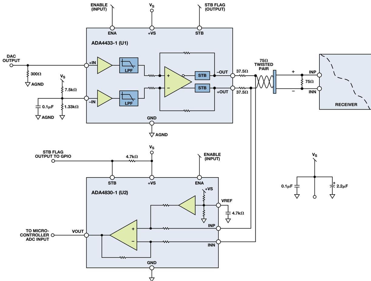
Figure 1. Wire diagnostic circuit using the ADA4433-1 (U1) and ADA4830-1 (U2).
