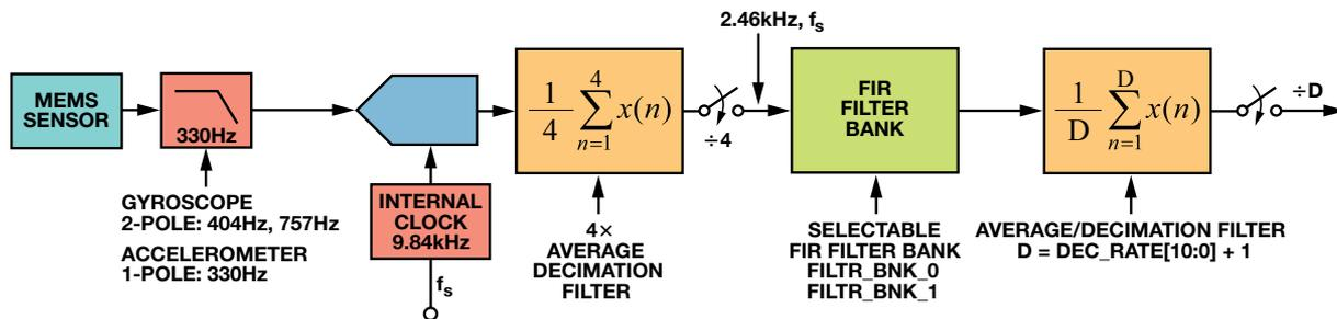
Figure 3. ADIS16488 sensor in a signal chain for frequency analysis.
