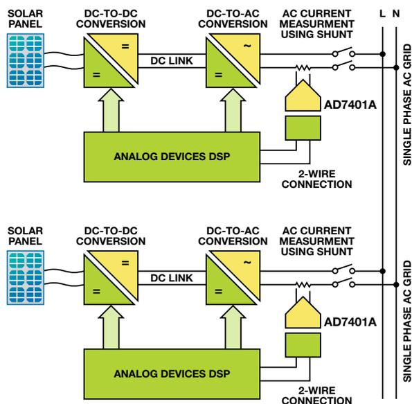
Figure 2. Solar PV system example.
