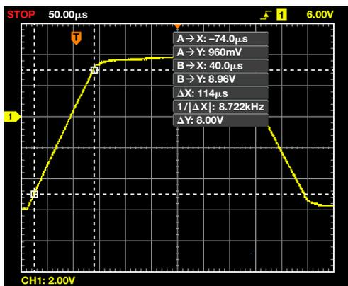
Figure 7. Rise time with 1-µF capacitive load.
