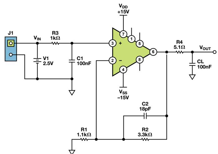
Figure 3. AD797 schematic design with gain = 4.
