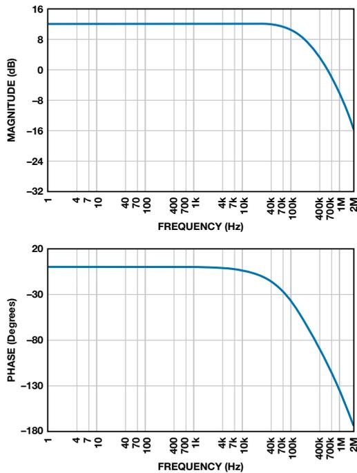
Figure 4. Frequency response of the AD797 with gain = 4.
