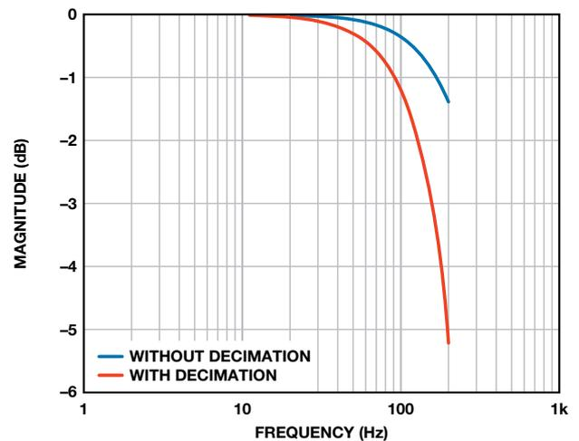
Figure 4. Analog filter and first decimation stage.
