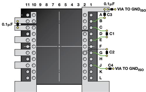
Figure 7. ADM3252E recommended printed circuit board layout.
