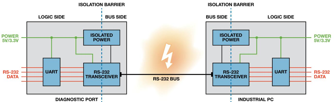
Figure 3. Isolated RS-232 interface.
