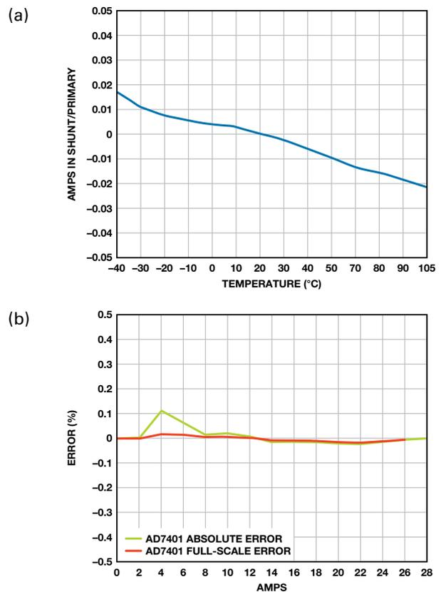
Figure 4. Offset and linearity of the AD7401A SMS solar module. a. Offset vs. temperature. b. Error vs. output current.
