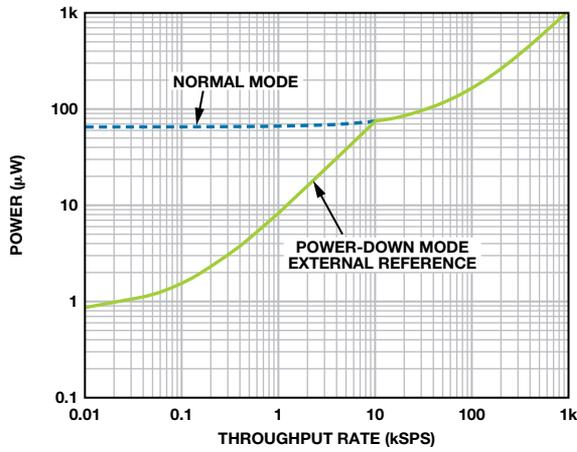
Figure 1. Power vs. throughput for the AD7091R ADC.
