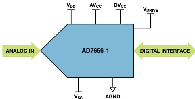
Figure 1. AD7656-1 connection diagram.
