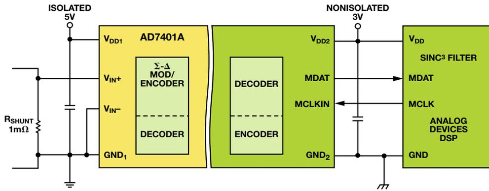
Figure 3. Isolated AD7401A ADC.
