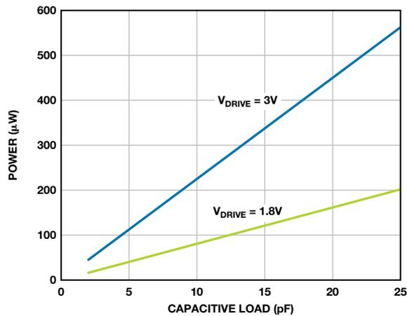
Figure 2. Typical interface power consumption vs. capacitive load.
