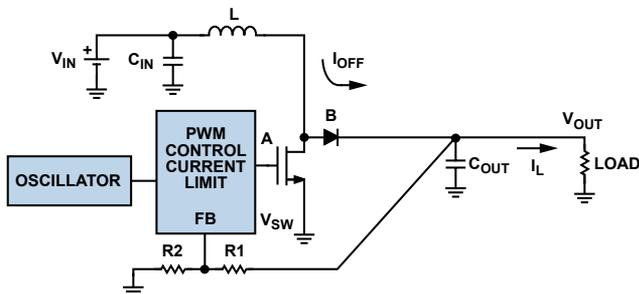
Figure 3. Boost regulator integrates oscillator, PWM control loop, and switching FETs.
