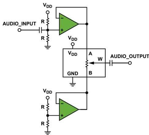
Figure 12. Single-supply ac signal conditioning.
