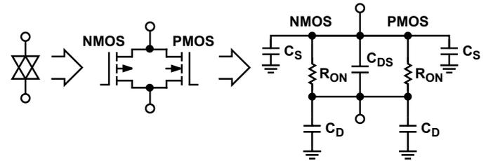
Figure 7. CMOS switch model.
