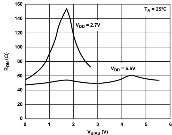
Figure 11. Switch resistance variation vs. supply voltage.
