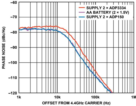
Figure 3. ADF4350 phase noise comparison at 4.4 GHz when powered with pairs of ADP3334 and ADP150 LDOs—and AA batteries.
