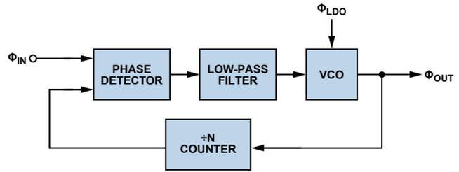
Figure 4. Small-signal additive VCO supply noise model.
