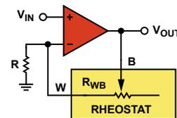
Figure 5. Noninverting amplifier in rheostat mode.
