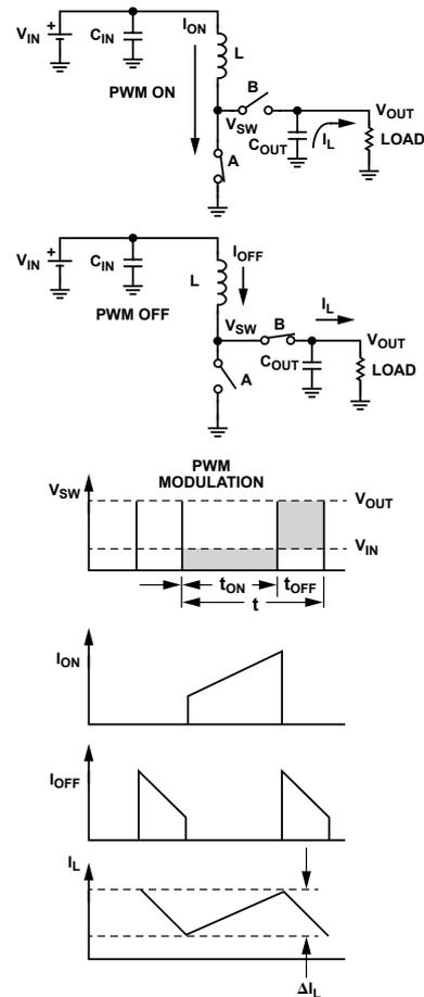
Figure 2. Buck converter topology and operating waveforms.
