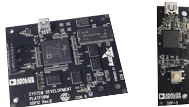
Figure 2. Controller boards: a) SDP-B. b) SDP-S.
