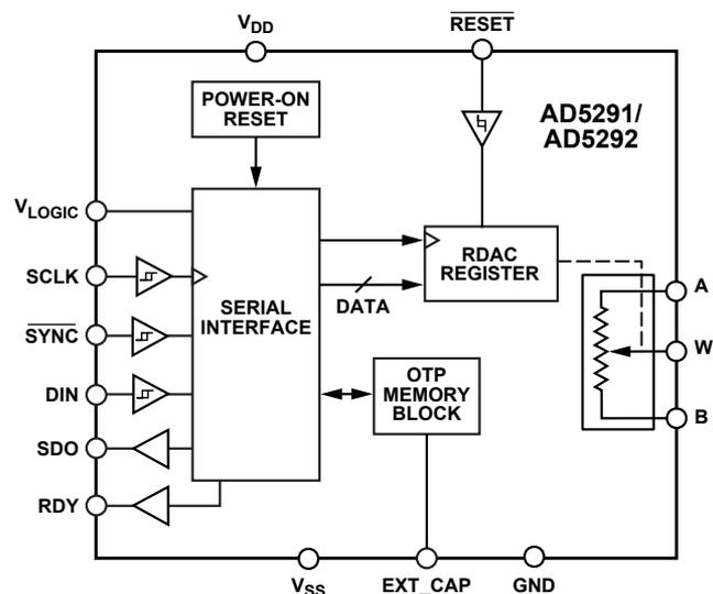
Figure 14. AD5291/AD5292 functional block diagram.
