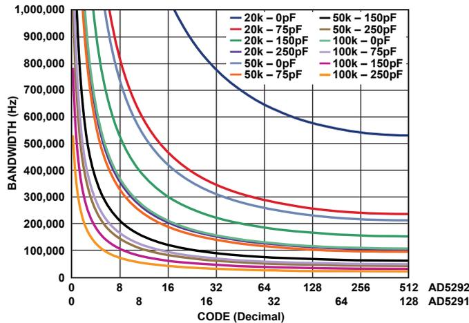
Figure 8. Maximum bandwidth vs. load capacitance for various resistance values.
