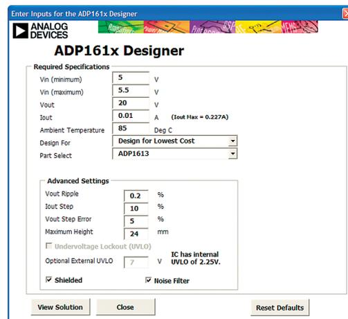
Figure 8. ADP1613 boost converter Excel design tool.
