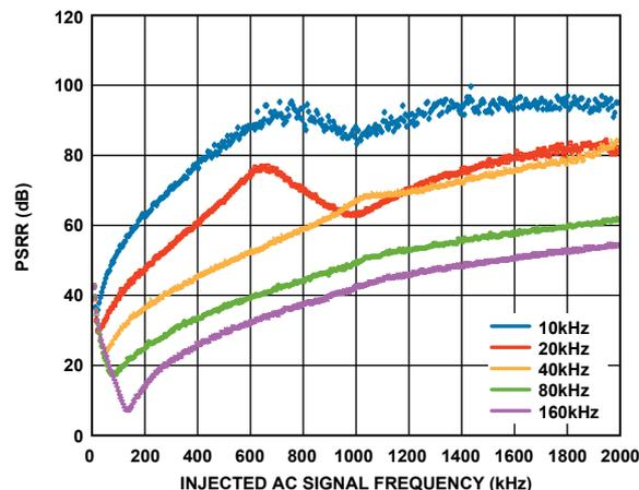
Figure 7. ADF4150HV charge pump power-supply rejection plot.
