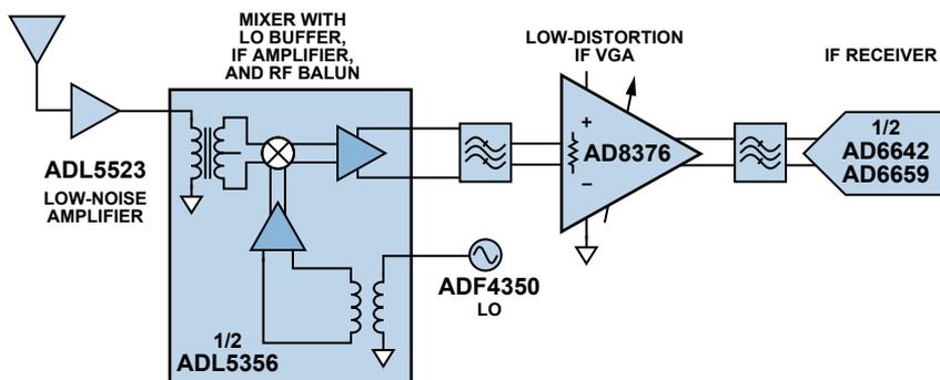
Figure 3. Superheterodyne receiver diagram; one channel shown.
