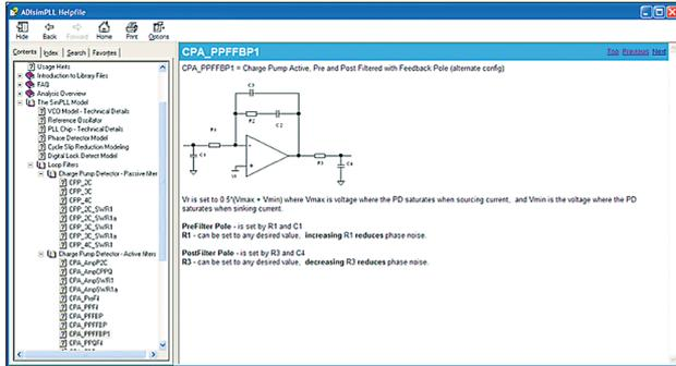
Figure 9. Screen view of CPA\_PPFFBP1 filter design in ADIsimPLL.
