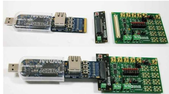
Figure 6. BeMicro SDK, interposer, and SDP controller.
