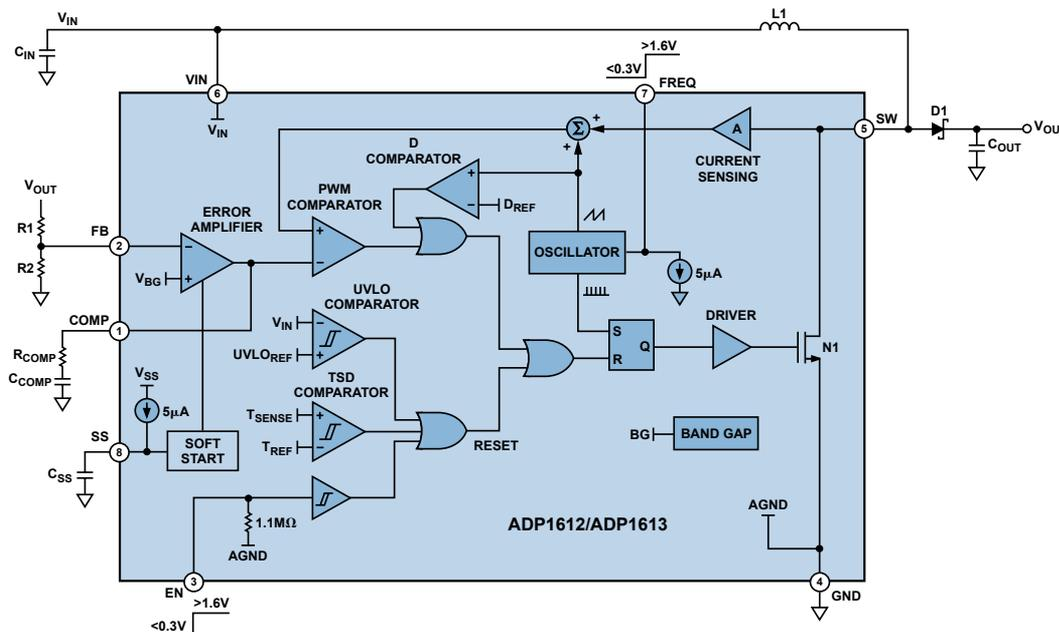
Figure A. ADP1612/ADP1613 functional block diagram.
