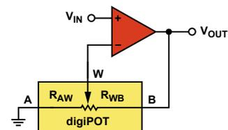
Figure 4. Noninverting amplifier in potentiometer mode.
