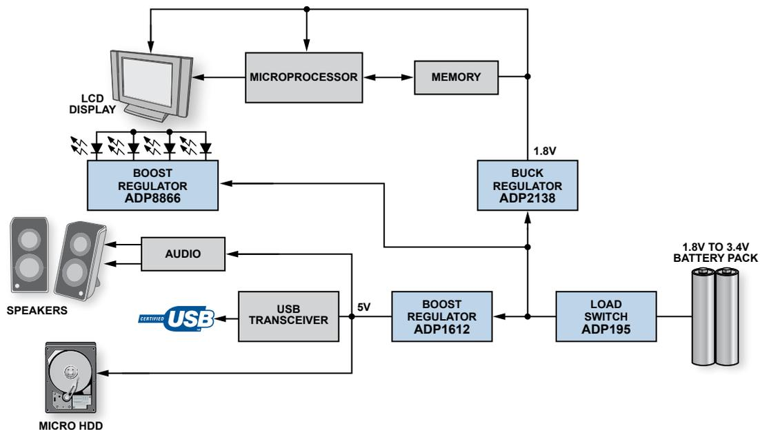
Figure 1. Typical low-power portable system.
