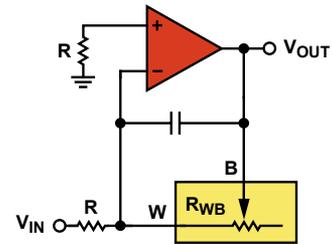
Figure 13. Adjustable amplification using a digiPOT with an inverting amplifier.
