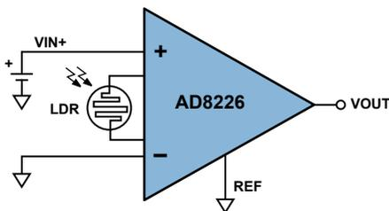
Figure 2. Simple circuit measures light intensity.
