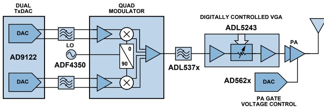
Figure 5. Transmitter diagram.
