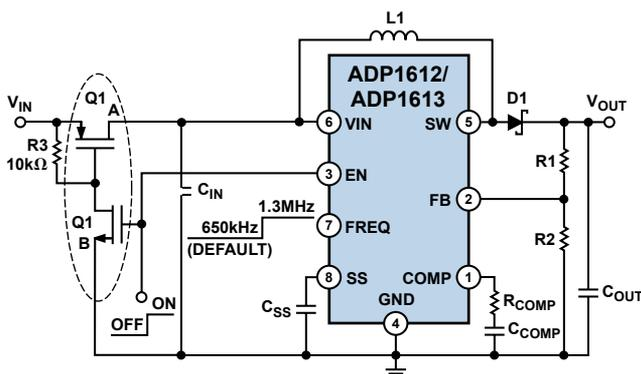
Figure 4. ADP1612/ADP1613 typical applications circuit.
