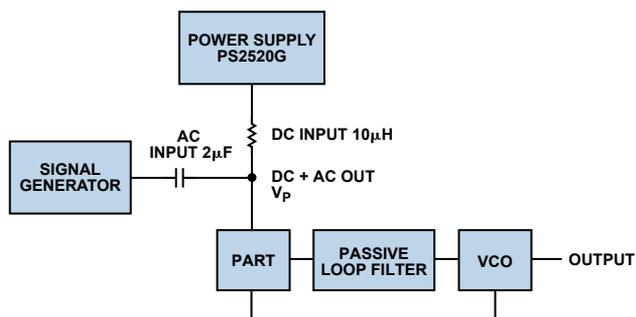
Figure 6. Setup for measuring charge pump power-supply rejection.
