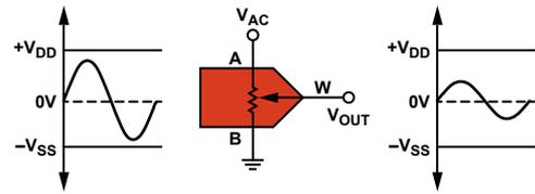
Figure 3. Signal attenuator.
