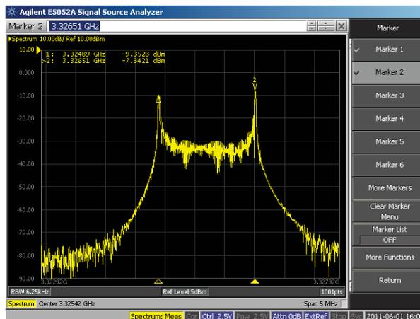
Figure 2. A spectrum-analyzer plot of ADF4350 VCO response to supply modulation by a 10-kHz, 0.6-V p-p square wave.
