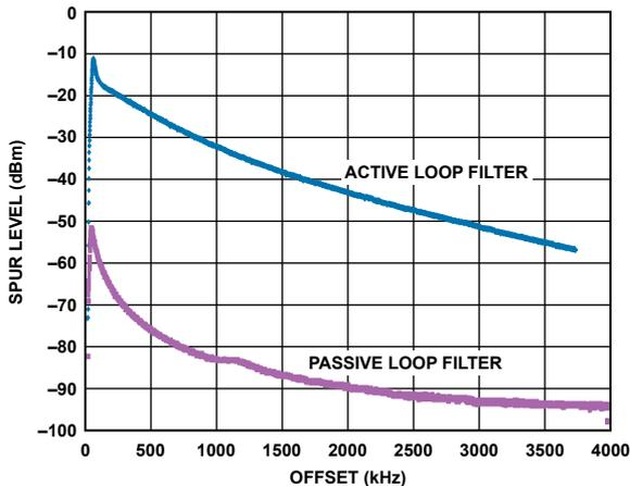
Figure 10. Power supply ripple level for active loop filter vs. high-voltage passive filter.
