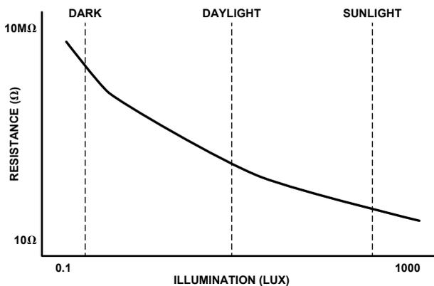
Figure 1. Sensor resistance vs. light intensity.
