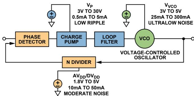
Figure 1. A basic phase-locked loop showing the various power-management requirements.
