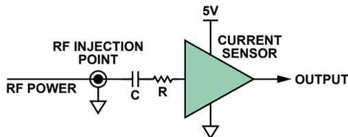
Figure 4. Direct power injection.
