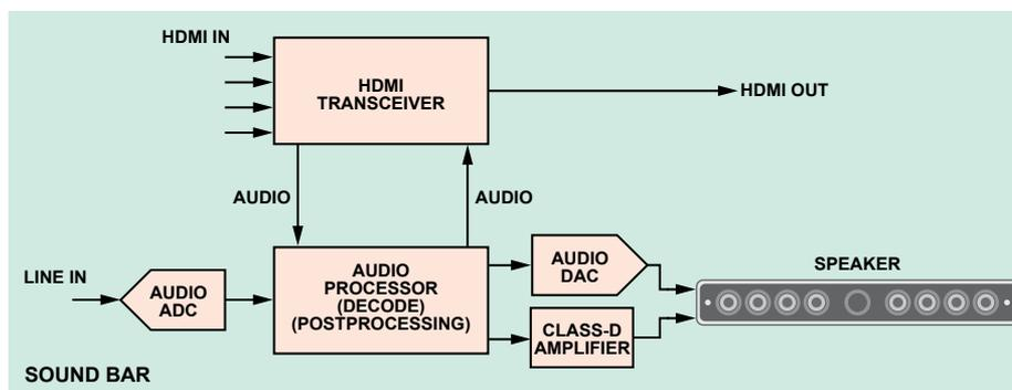
Figure 3. Block diagram of a typical sound bar with HDMI hub.
