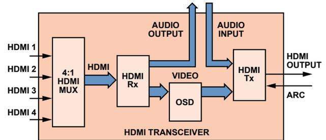
Figure 1. Functional block diagram of an HDMI transceiver.
