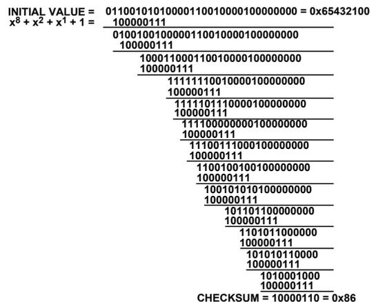
Figure 2. Generating a checksum for a 24-bit number (0x654321).
