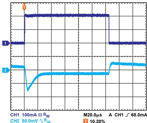
Figure 2. Transient response with  $C_{OUT} = 10 \mu\text{F}$ .
