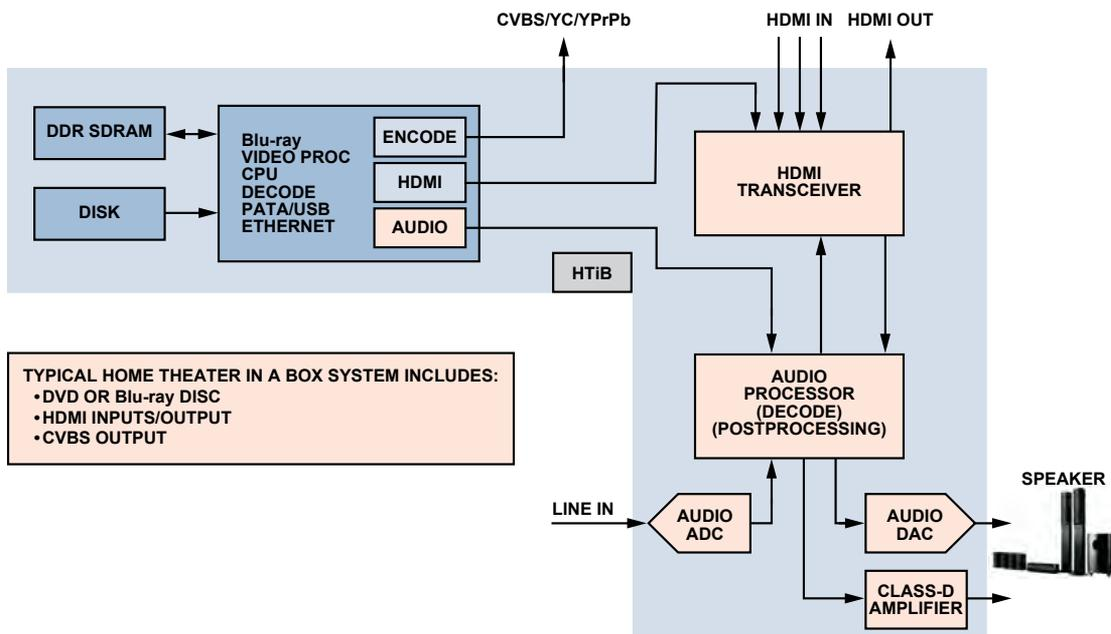
Figure 2. Block diagram of a typical HTiB system.
