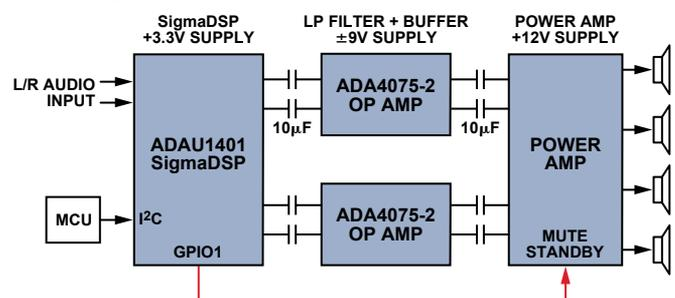
Figure 3. Automotive audio system with four speakers.
