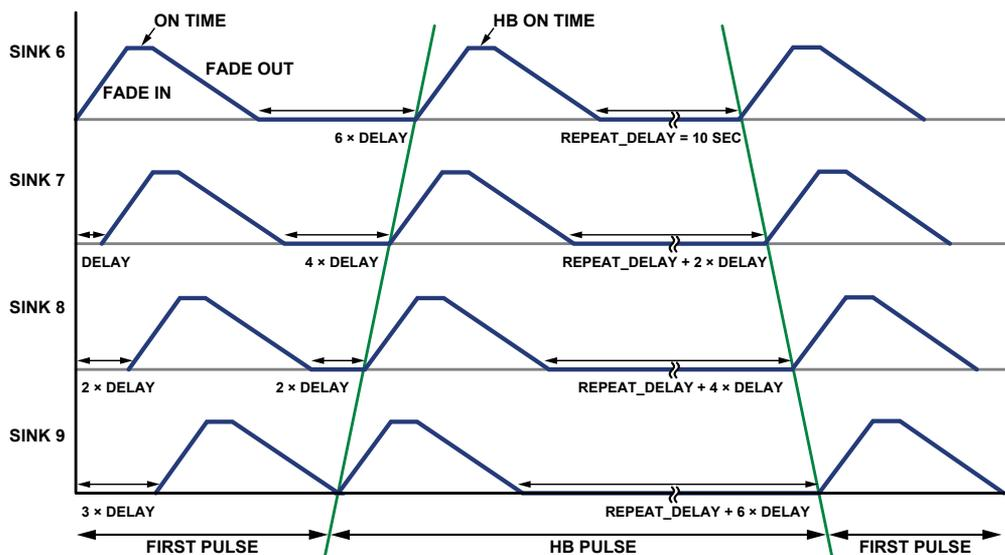
Figure 4. Four-channel dynamic indicator display.
