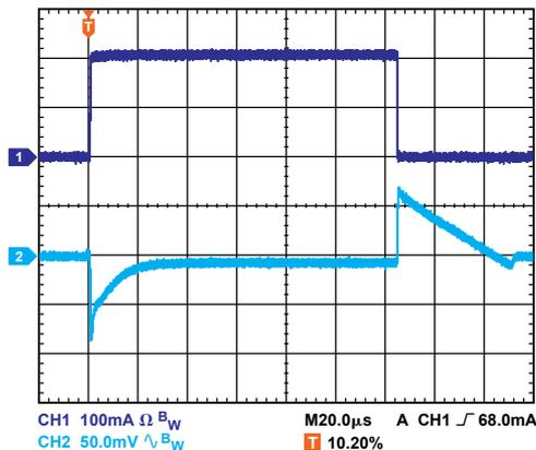
Figure 1. Transient response with  $C_{OUT} = 1 \mu\text{F}$ .
