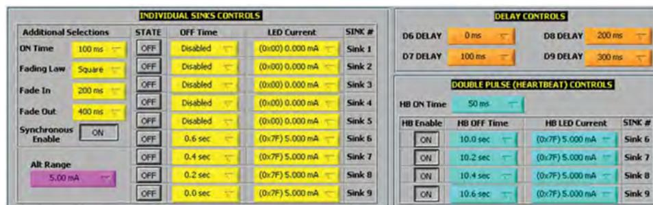
Figure 5. ADP8866 graphical user interface for programming dynamic indicators.
