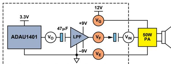
Figure 1. Example of noise sources in an automotive audio system.
