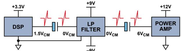
Figure 2. The concept of how pop noise is created in the speaker.
