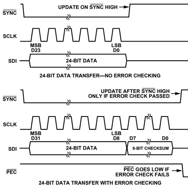
Figure 1. SPI write with and without packet error checking.
