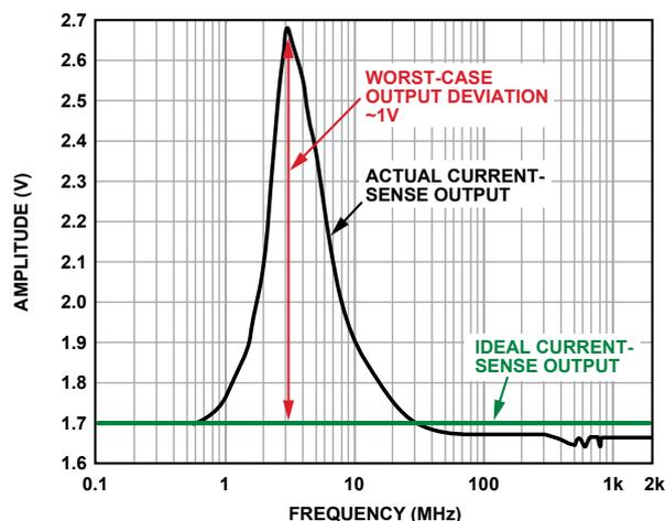
Figure 2. Output of current sensor with no internal EMI filters (forward power = 12 dBm, 100 mV/division, peak dc output at 3 MHz).
