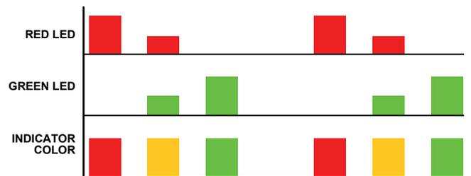
Figure 2. Red and green blinking pulse sequence with resulting colors.
