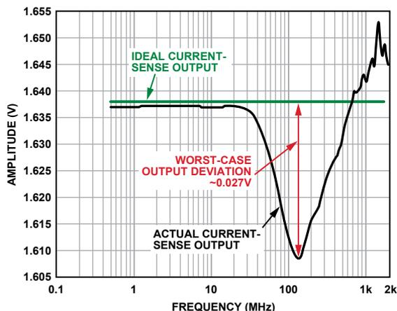
Figure 3. Output of current sensor with internal EMI filters (forward power = 12 dBm, 5 mV/division, peak dc output at >100 MHz).
