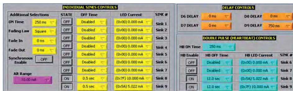
Figure 3. ADP8866 graphical user interface for programming indicator LEDs.
