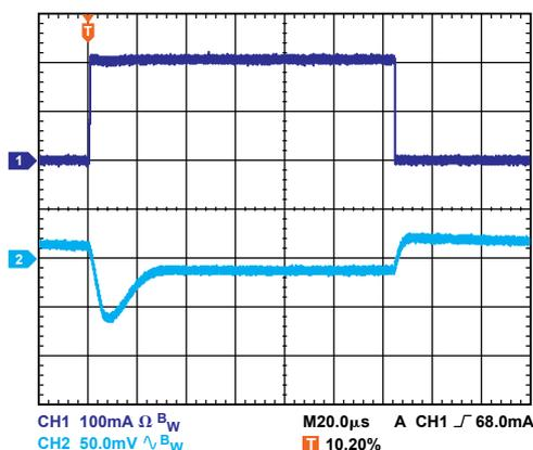
Figure 3. Transient response with  $C_{OUT} = 20 \mu\text{F}$ .
