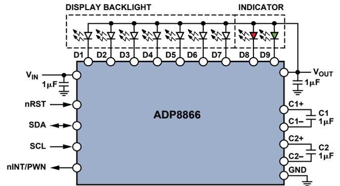
Figure 1. The ADP8866 is set up to control backlight illumination and indicator LEDs.
