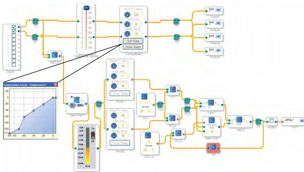
Figure 4. SigmaStudio schematic for rms detection, GPIO control, and compression.
