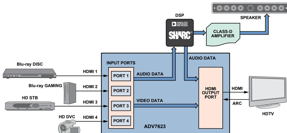
Figure 4. HTiB system using the ADV7623 HDMI transceiver.
