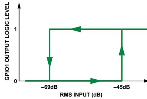
Figure 5. RMS threshold settings and the relationship between input and output.
