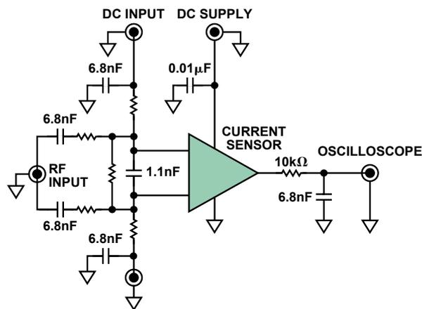
Figure 5. Schematic for EMI susceptibility testing.
