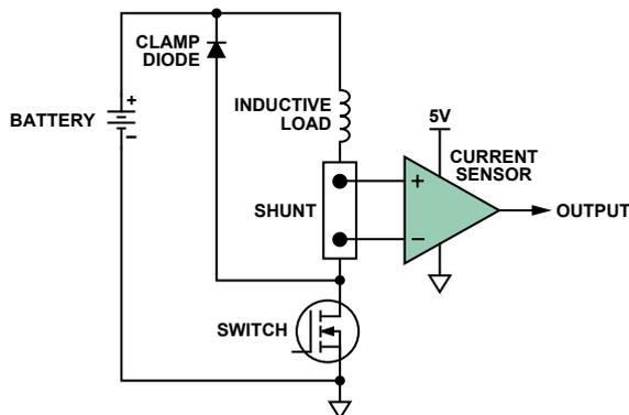
Figure 1. High-side current monitoring.
