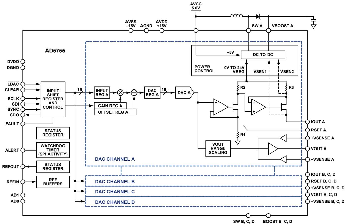
Figure A. Functional block diagram of the AD5755 quad DAC. All four channels are identical.
