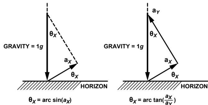
Figure 3. MEMS tilt sensor operation.
