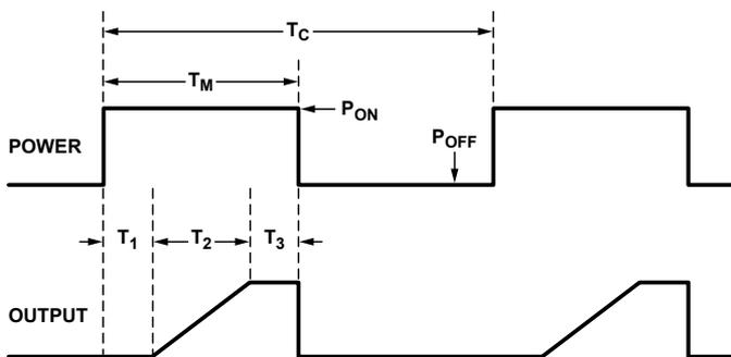
Figure 2. Sensor response during power cycling.
