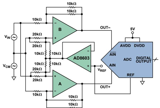
Figure 2. Differential amplifier drives ADC.
