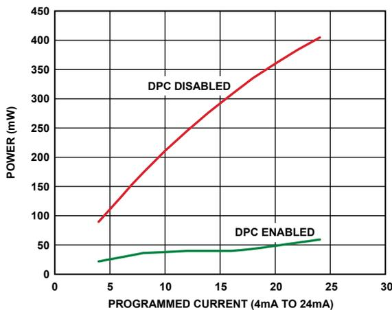
Figure 6. Dissipation comparison with and without dynamic power control.
