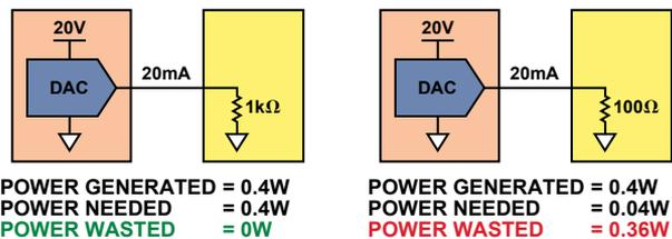
Figure 3. Power is wasted when full-scale output is much less than the power-supply voltage.
