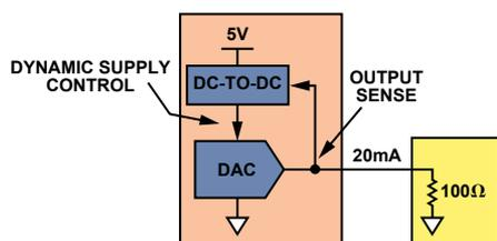
Figure 4. Dynamic supply control principle.
