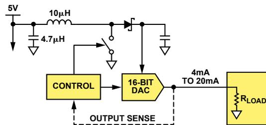
Figure 5. Voltage boost with power control.
