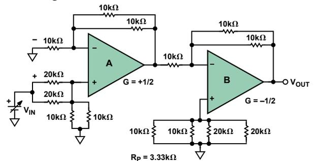
Figure 3. Connection for gains less than 1.
