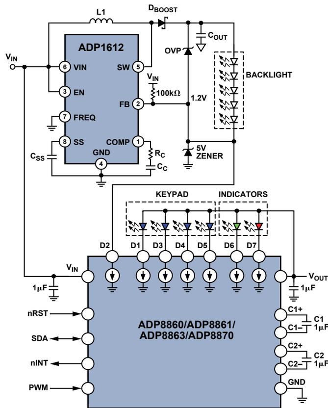
Figure 1. ADP1612 boost converter and ADP8860 LED driver implement programmable drive for backlight and auxiliary LEDs.
