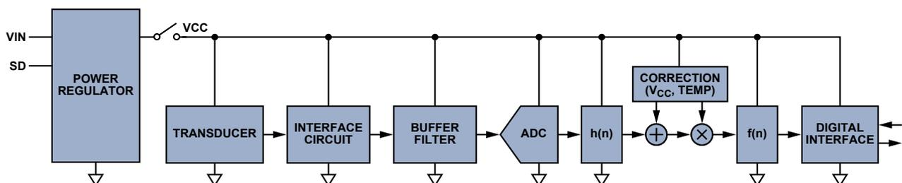
Figure 1. Example of a sensor system.
