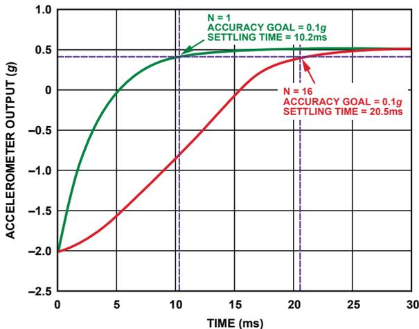
Figure 5. Power-on transient response.
