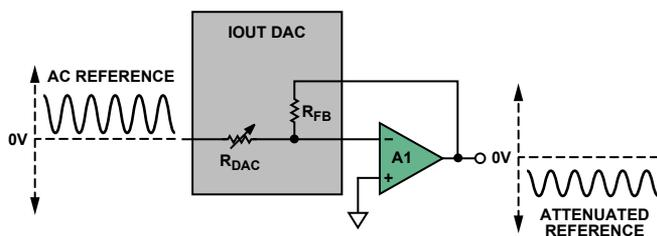
Figure 1. Inverting gain configuration.
