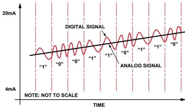
Figure 9. HART signal riding on an increasing loop current.
