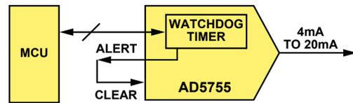
Figure 7. Watchdog timer flags loss of control signal and returns DAC to clear setting.
