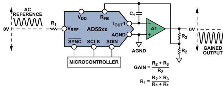
Figure 3. Increasing the gain of a multiplying DAC.
