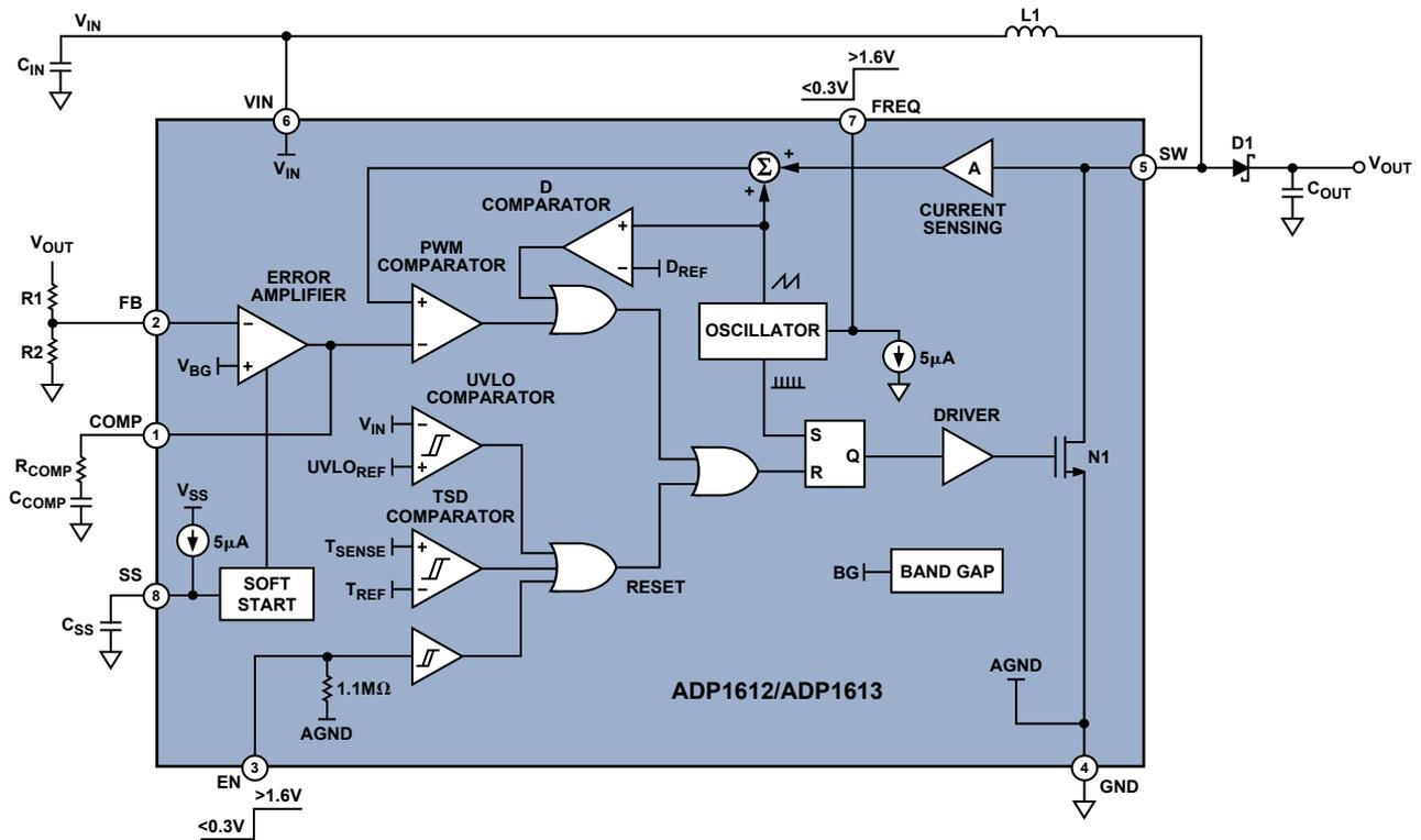
Figure 2. ADP1612/ADP1613 block diagram.
