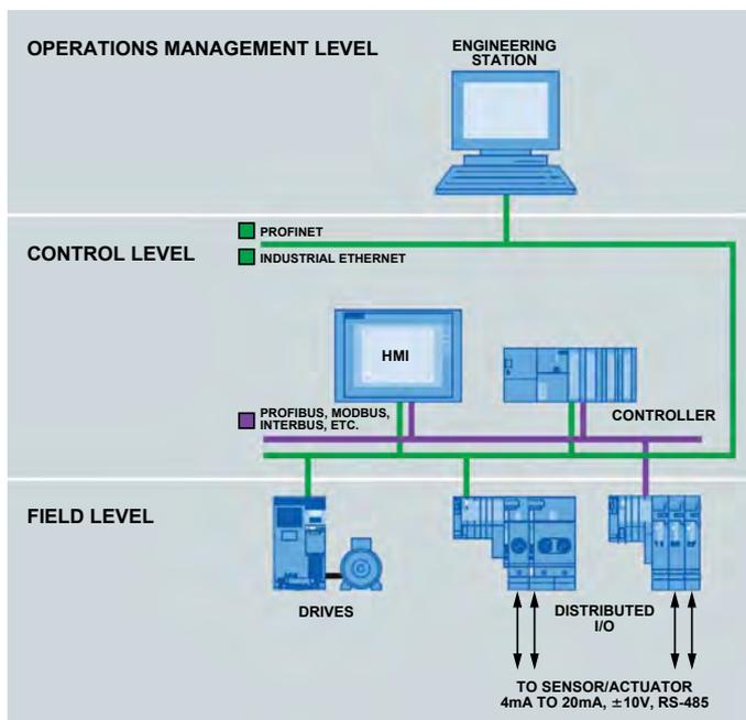
Figure 1. Hierarchy in a control system.
